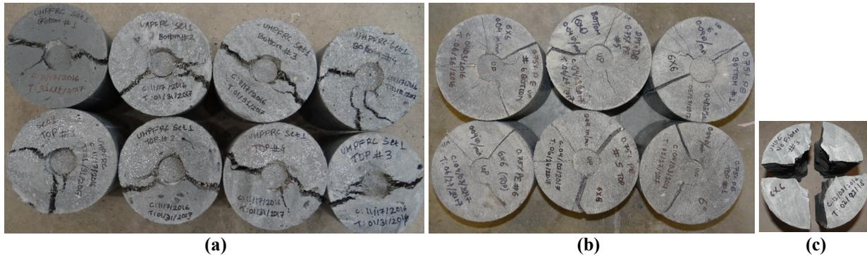
Figure 4. Crack patterns in DPT specimens (a) UHP-FRC with steel fibers, (b) UHP-FRC with PE fibers, and (c) UHPC (0% fibers)
