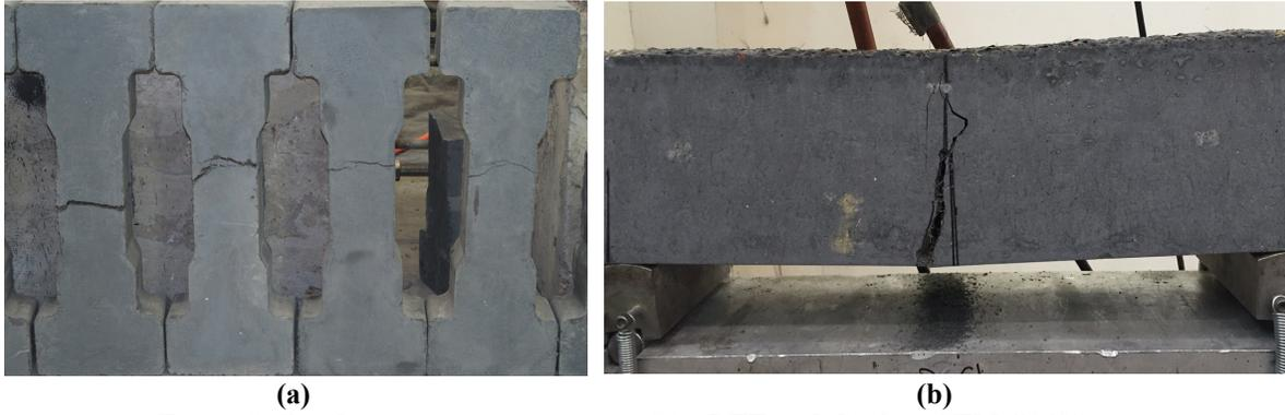
Figure 3. Crack patterns in specimens of (a) DTT and (b) the ASTM C1609 test
