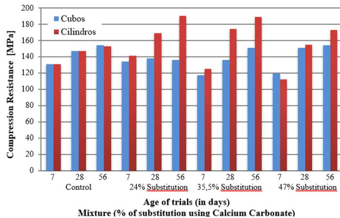
Figure No. 6 Results of compression resistance in 7, 28 and 56 days trial period for all mixtures.
