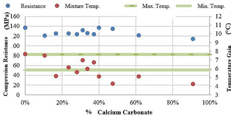
Figure No. 2 Resistance & Maximum Temperature Gain vs % Carbonate
