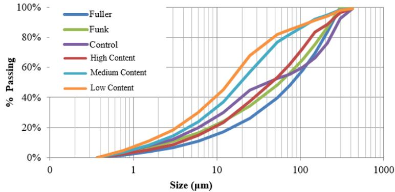
Figure No. 5 Compactness slope curves of tested mixtures.
