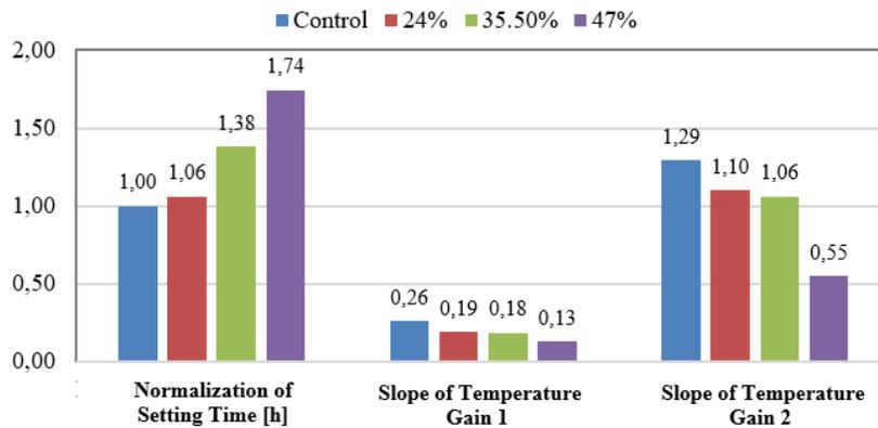
Figure No. 4 Mixture properties according to calcium carbonate content.
