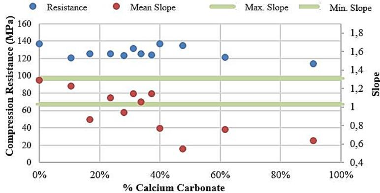
Figure No. 3 Resistance & Slope vs % of Carbonate.
