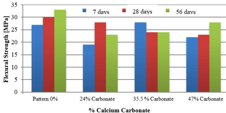
Figure No. 8 Results of Flexural Strength after 7, 28 and 56 days for all mixtures tested.
