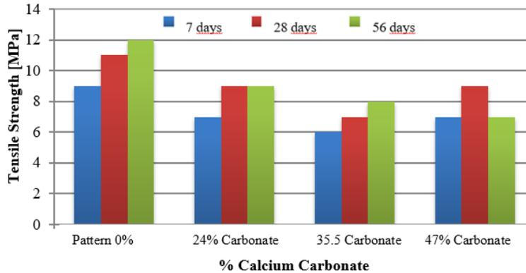
Figure No. 9 Results of tensile strength for 7, 28 and 56 day mixtures.
