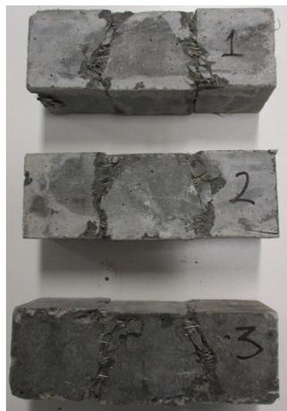
Figure 7. Double Shear Failure Mode of Direct Shear Test Specimens.
