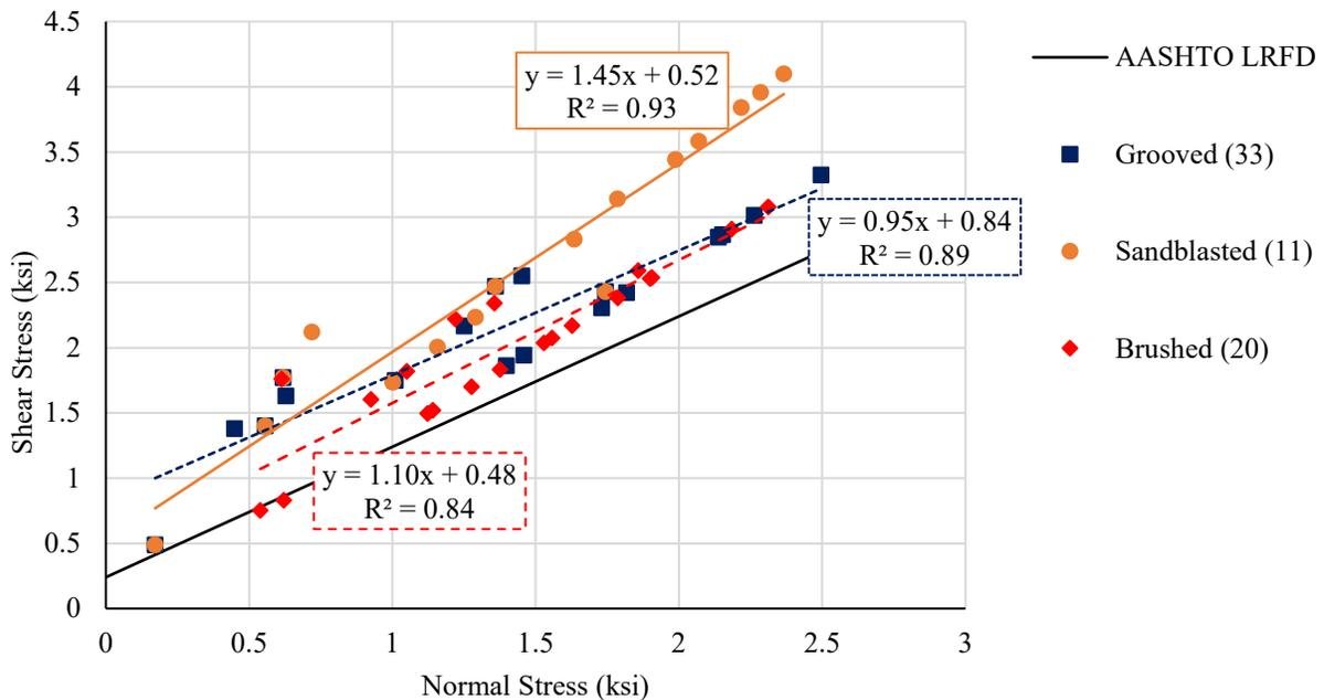
Figure 3. Interface Shear Resistance of CC-UHPC with Different Surface Textures (1 ksi = 6.9 MPa).
