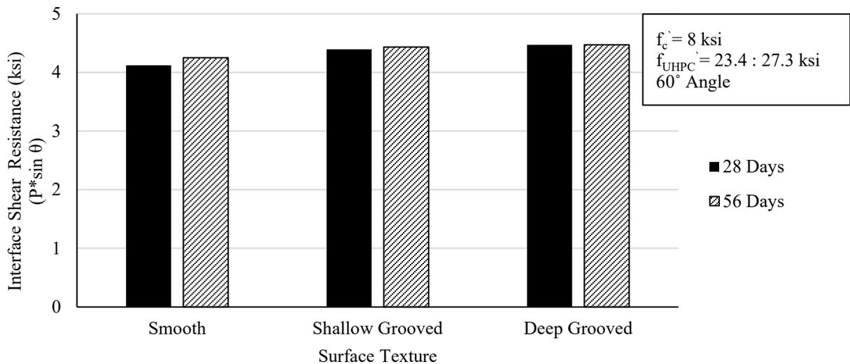
Figure 9. Interface Shear Resistance of CC-UHPC at 28 and 56 Days for Different Surface Textures (1 ksi = 6.9 MPa).
