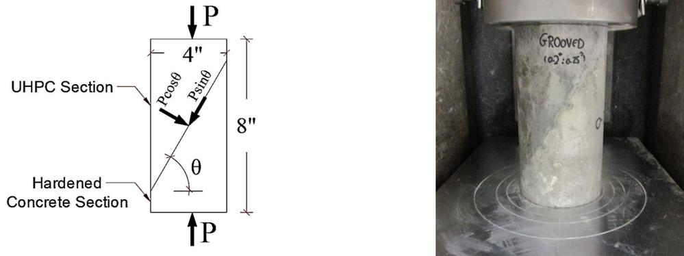
Figure 6. Slant Shear Test Specimen Dimensions and Test Setup (1 in. = 2.54 cm).
