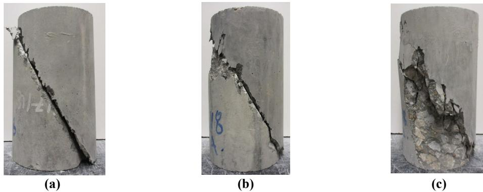
Figure 8. Slant Shear Specimen Failure Modes; a) Bond Failure, b) Bond Failure and CC Fracture, and c) CC Failure.
