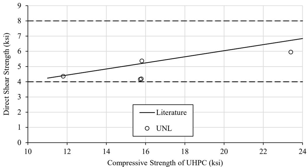
Figure 10. Results of Direct Shear Test and their Comparison to the Literature (1 ksi = 6.9 MPa).
