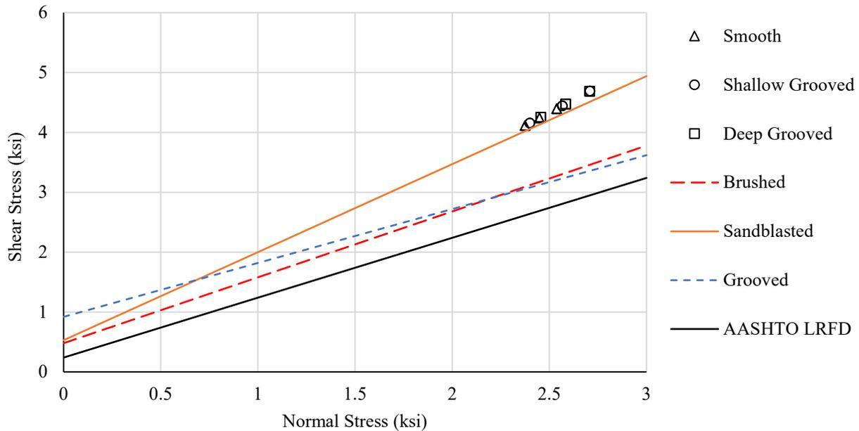
Figure 11. Results of Slant Shear Test and their Comparison to the Literature (1 ksi = 6.9 MPa).
