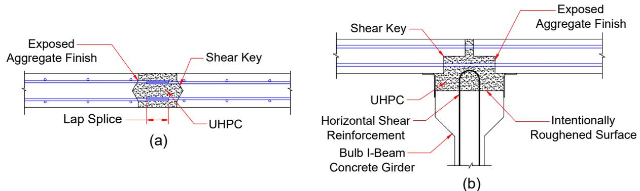
**Figure 1: Examples of UHPC Field-Cast Bridge Connections: (a) Deck Panel-to-Panel Connection, and (b) Deck Panel-to-Girder Connection (Graybeal 2014).**
