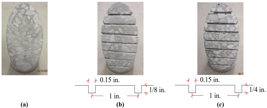
Figure 5. Interface Textures of Hardened Conventional Concrete; (a) Smooth, (b) Shallow Grooved, and (c) Deep Grooved (1in. = 2.54 cm).
