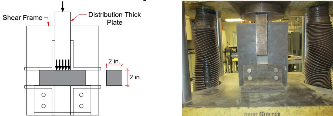
Figure 4. Direct Shear Test Setup (1 in. = 2.54 cm).
