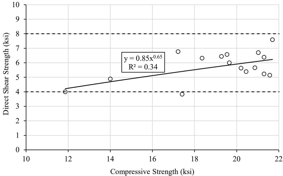
Figure 2. UHPC Direct Shear Strength as Function of its Compressive Strength (1 ksi = 6.9 MPa).
