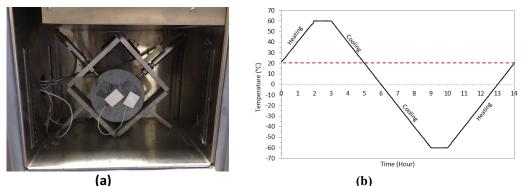
Figure 2. (a) OCD Test Setup; (b) Temperature Profile used in The Test
