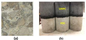
Figure 1. Specimens Preparation: (A) An Exposed Surface; (B) Composite Specimens
