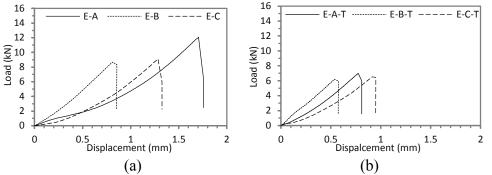
Figure 5. Load Versus Displacement Plots Under Direct Tension: (a) Without Temperature; (b) With Temperature
