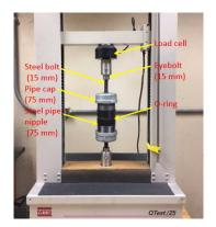
Figure 3. Testing Machine with Composite Specimen
