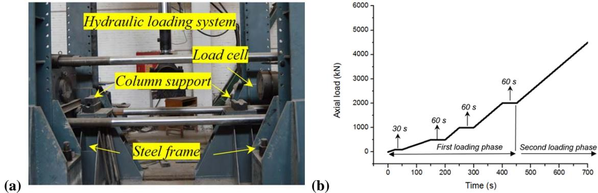
**Figure 4. Axial load-carrying capacity testing system and load sequence**
