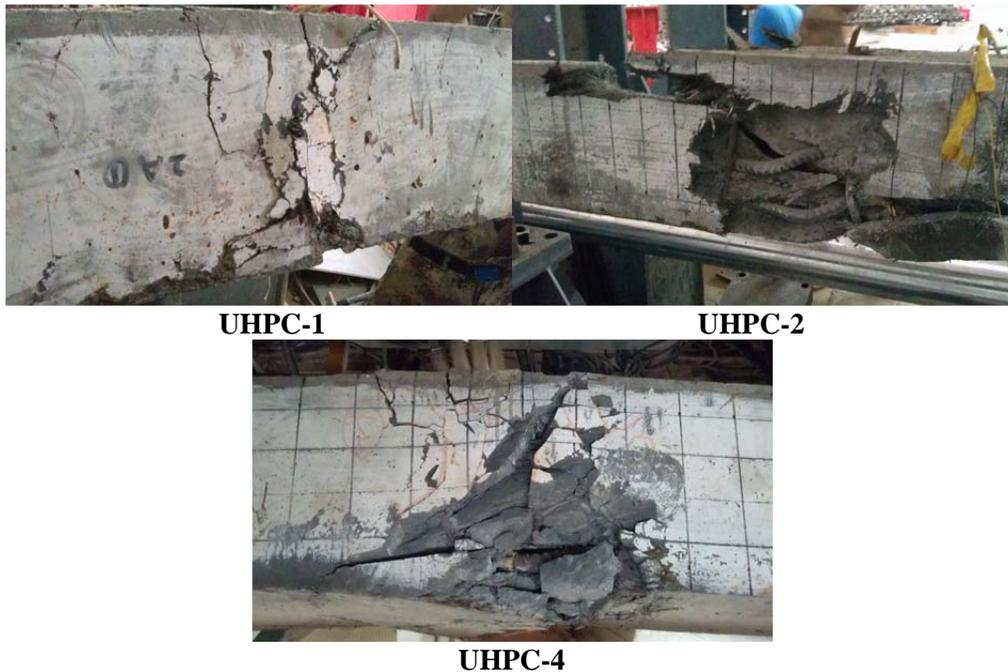
Figure 6. UHPC columns after residual loading test
