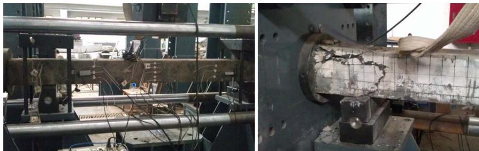
**Figure 5. End concrete crushing of undamaged (non-blast tested) UHPC column**
