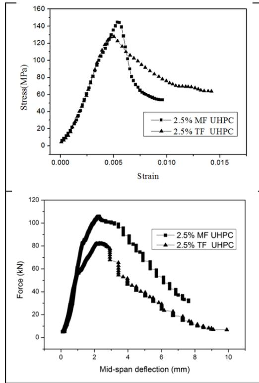
**Figure 1. Compressive stress-strain and flexural bending force-displacement curves of UHPC**
