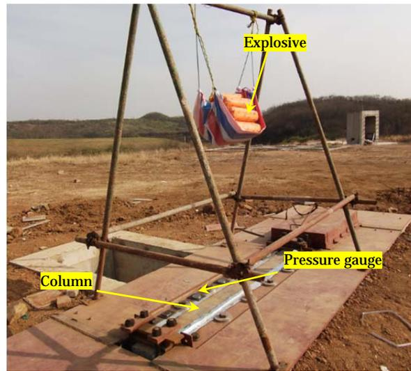
**Figure 2. Field test setup**
