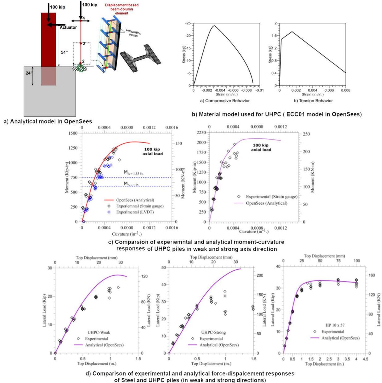
**Figure 7: Fiber based analytical model and comparison of experimental and analytical results**
