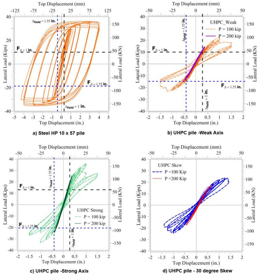
**Figure 5: Force - displacement response of Steel and UHPC piles under cyclic loading**
