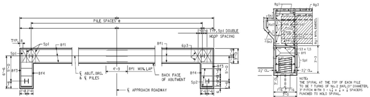
Figure 3: Standard details of pile-to-abutment connection used by IowaDOT
