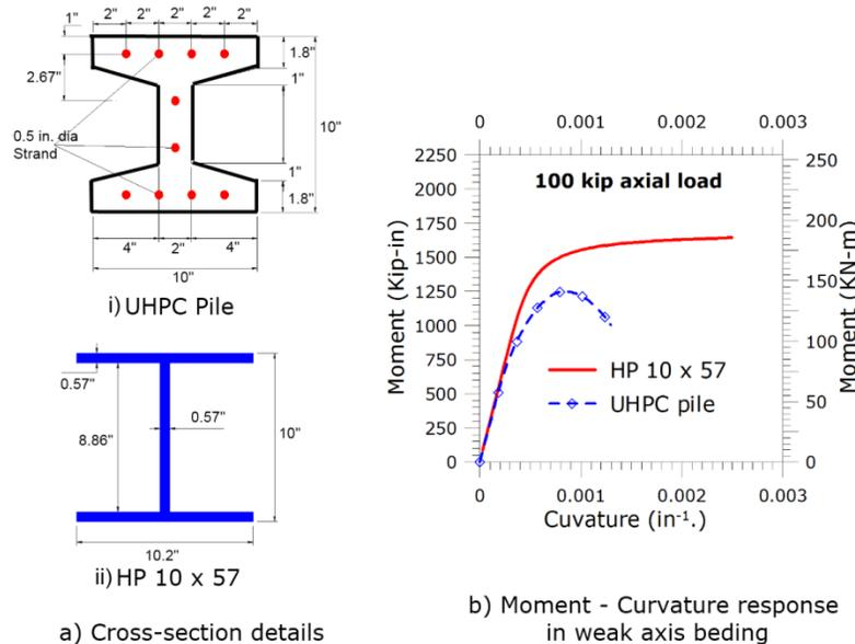
**Figure 1: Comparison between UHPC prestressed pile and standard steel HP 10 x 57 pile.**
