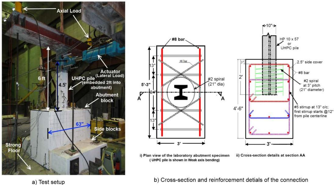
**Figure 4: Details of the pile-to-abutment connection tests**
