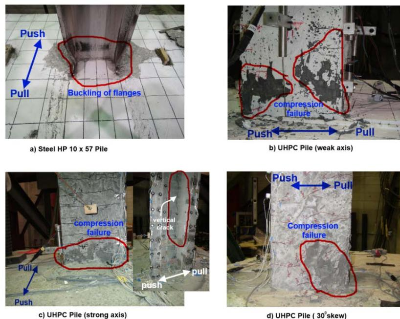
**Figure 6: Observed damage in piles at failure.**
