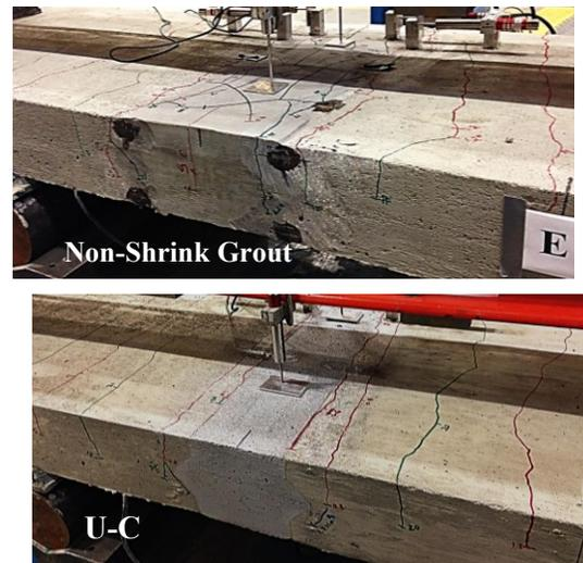
Figure 6. Cracking in the Connection Region after Cracking and Fatigue Cycles
