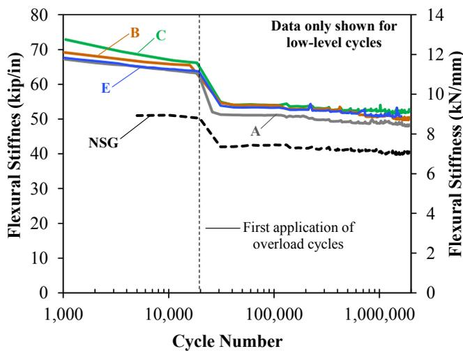
Figure 5. Degradation of Flexural Stiffness During Fatigue Loading
