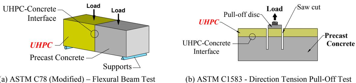
Figure 1. UHPC-to-Precast Concrete Bond Test Configurations
