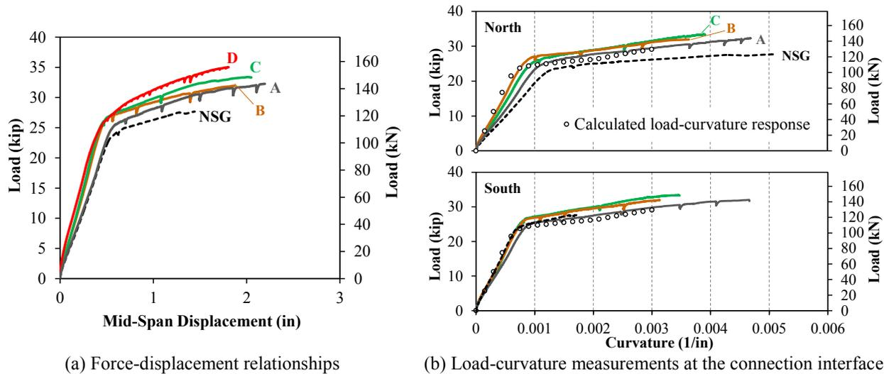
Figure 7. Ultimate Loading Response of Deck Panel Specimens (1 in. = 25.4 mm)
