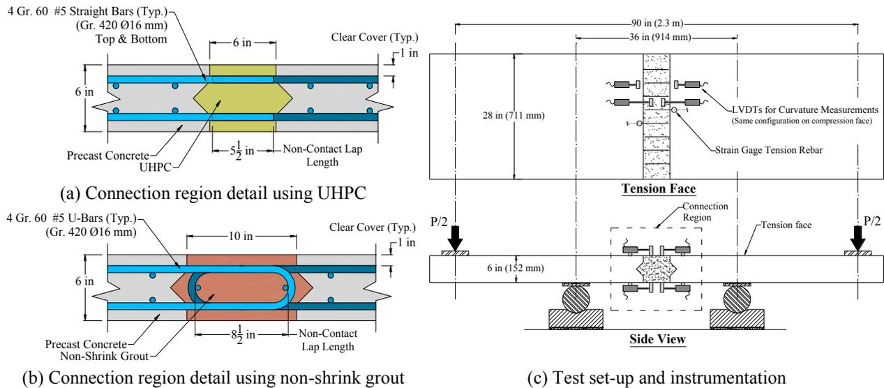
Figure 2. Specimen Details (1in = 25.4mm)
