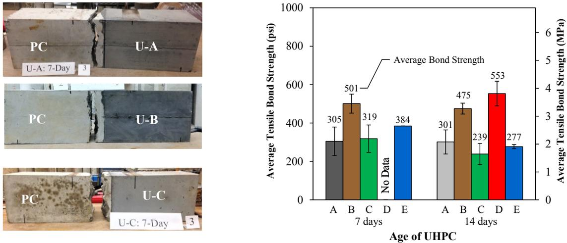
(a) Photos from flexural beams tested at 7-days (b) Bond strength as measured by direct tension pull-off testing
