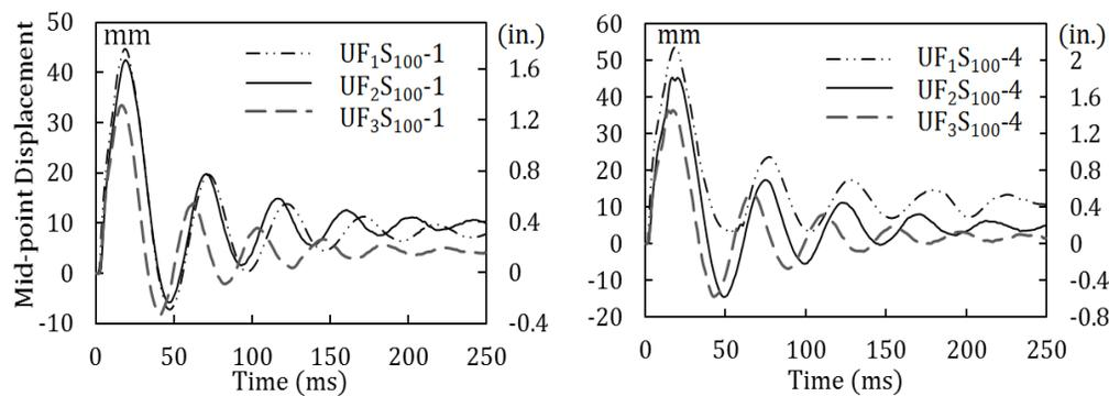
Figure 5. Influence of fiber content on mid-point displacement (left: 1<sup>st</sup> test; right: 4<sup>th</sup> test)
