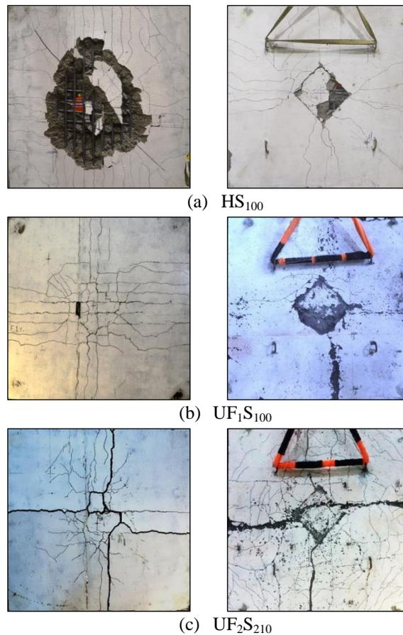
Figure 2. Final crack patterns (left: bottom surface; right: top surface)
