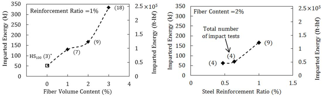
Figure 3. Impact capacities of HSC and UHPFRCs plates
