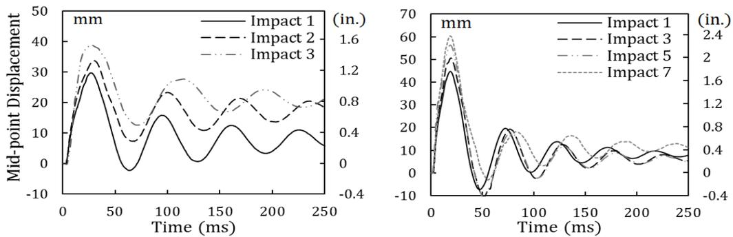
Figure 4. Mid-point displacement-time histories for plates (left: HS<sub>100</sub>; right: UF<sub>1</sub>S<sub>100</sub>).
