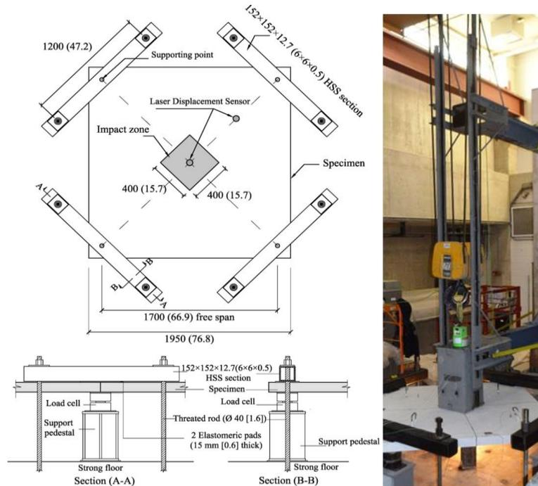
Figure 1. Drop-weight impact test setup (dimensions in mm[in.]) (Othman and Marzouk)
