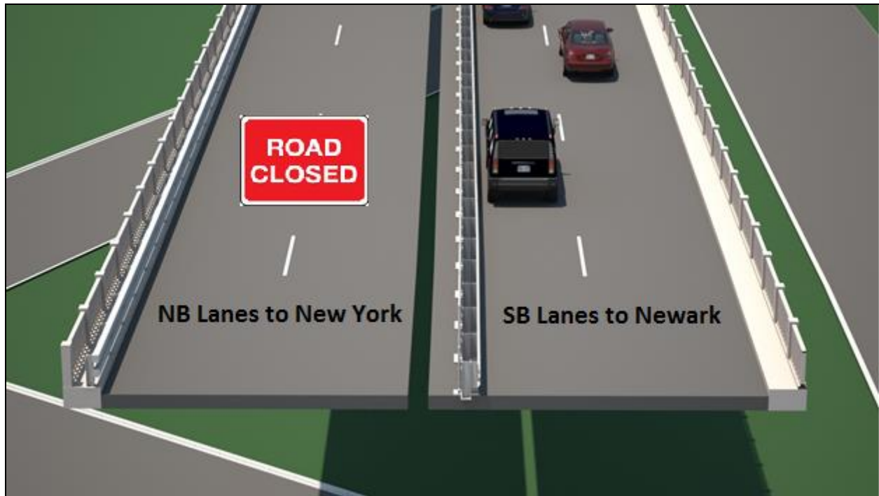
Figure 6. Temporary Lane Arrangement for Northbound Redecking
