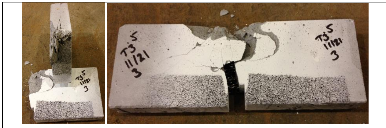
Figure 5. Examples of CS-0.5% specimen with crushing failure test using M-SEFIM with Type 3 coupler
