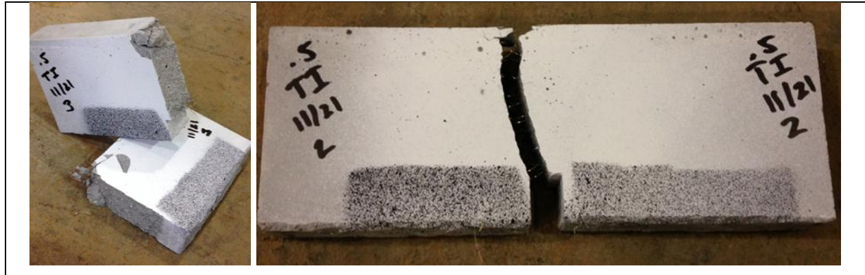
Figure 4. Examples of CS-0.5% specimen after testing using M-SEFIM with Type 1 coupler
