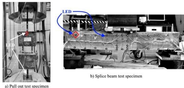
**Figure 3 LED layout used on test specimens during Phase-I and Phase-II testing**
