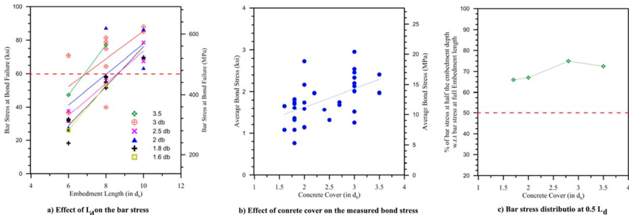
Figure 5 summary of experimental results from the pull out testing.
