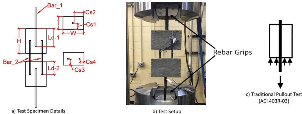
**Figure 1 Pullout test specimen and test setup details.**
