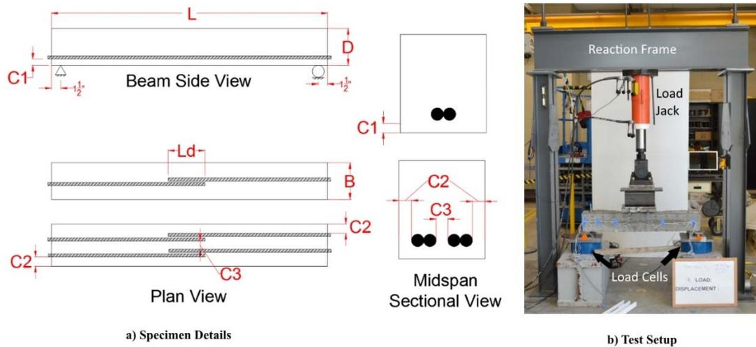
**Figure 2 Beam splice test details (Phase-II testing).**
