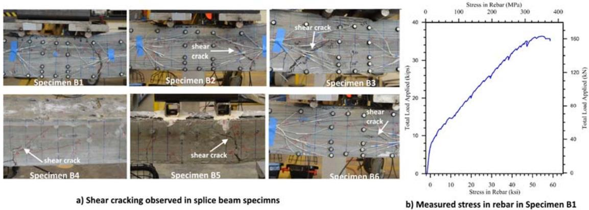
**Figure 6 Shear cracking and measured rebar stress in beam splice specimen.**
