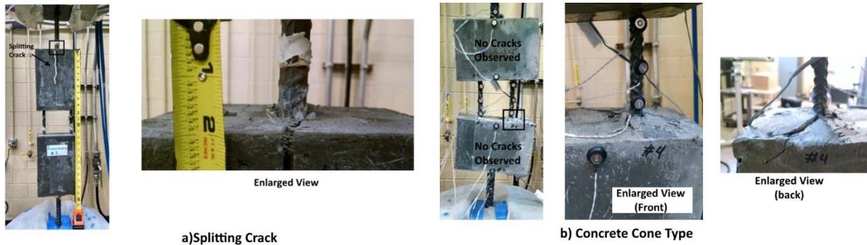
Figure 4 Failure mechanisms observed in pull out test specimens.
