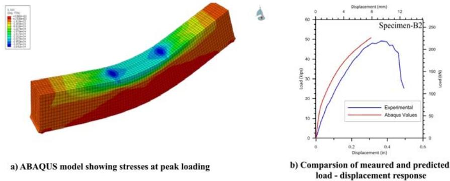
**Figure 7 ABAQUS modelling and comparison of load-displacement response**
