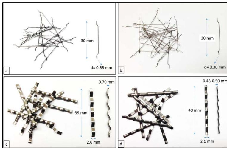
Figure 3. Existing fibers dimensions: a) kinked carbon steel, b) kinked stainless steel, c) undulated stainless steel, d) undulated carbon steel.
