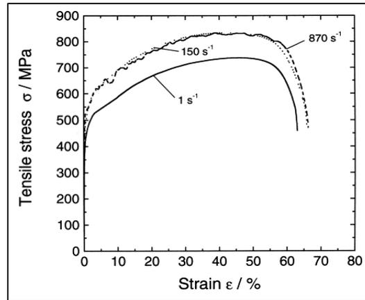
Figure 2. Influence of strain rate on stress vs. strain behavior of TWIP steel (from [6]).
