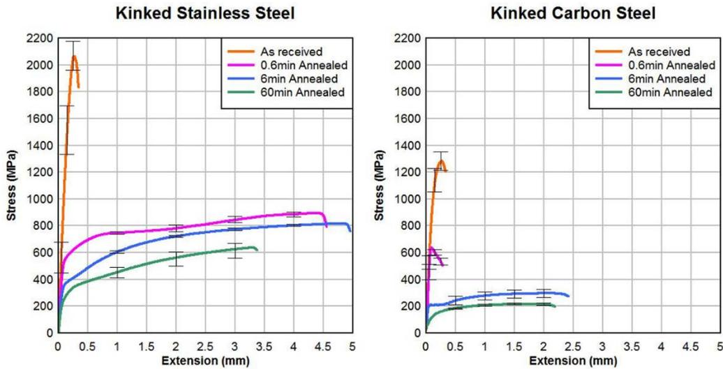
**Figure 7. Mechanical comparison of fiber including heat treatment.**
