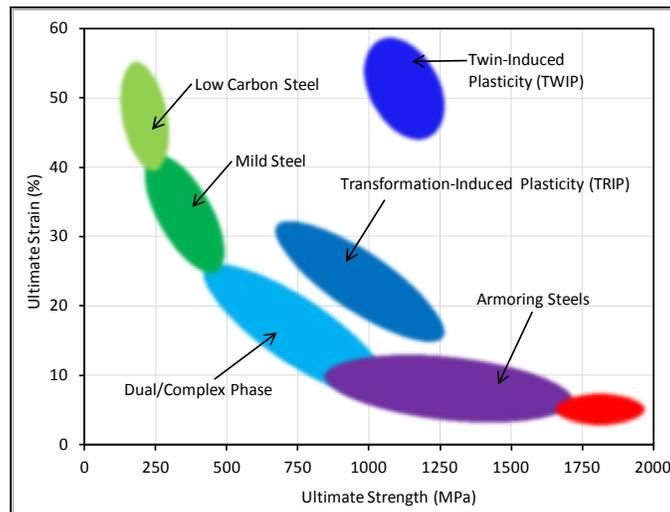
**Figure 1. Comparison of ultimate strain vs. ultimate strength for various families of metallic materials (from [9]).**
