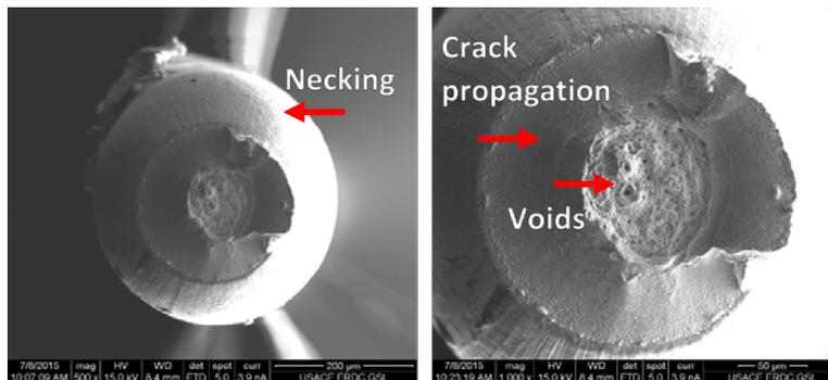
**Figure 9. Kinked stainless steel fiber fractography.**
