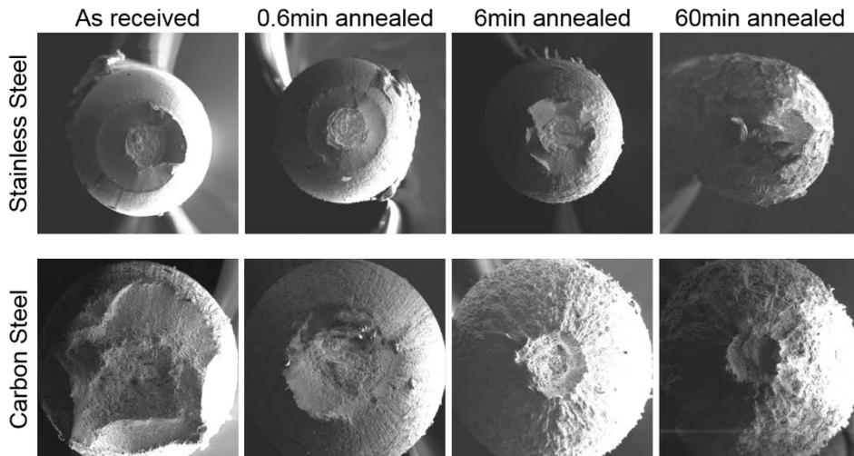
**Figure 10. Fracture surface as annealed increment.**
