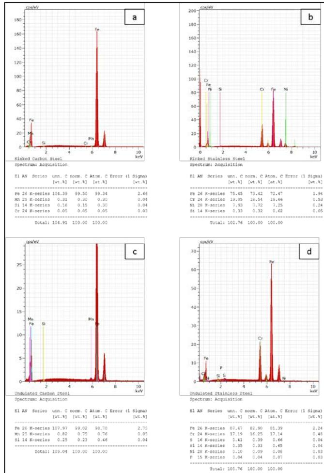
**Figure 5. EDX results for: a) kinked carbon steel, b) kinked stainless steel, c) undulated carbon steel, d) undulated stainless steel.**
