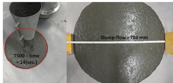
**Figure 1:** The slump-flow test of UHPFRC\_4mm with 1.5 Vol.-% StF1 ( $L_{f1}/D_{f1} = 13\text{mm}/0.2\text{mm}$ ). The results of  $T_{500}$  – time = 14 seconds (left), and slump-flow = 780 mm (right).
