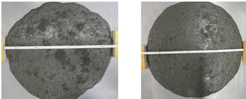
**Figure 5:** Fibres clumping (and balling) in the UHPC\_8mm – 0.75 Vol.-% StF2 (left) and in the UHPC\_2.5mm – 1.75 Vol.-% StF1 (right). Although these fibre concretes have the slump-flow of 650 mm and 700 mm, respectively, they cannot be used in practice.
