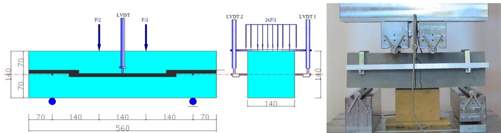
Figure 3: Four-point bending tests on unnotched beam of 140x140x560 mm<sup>3</sup> according to the ASTM C1609/C1609M.
