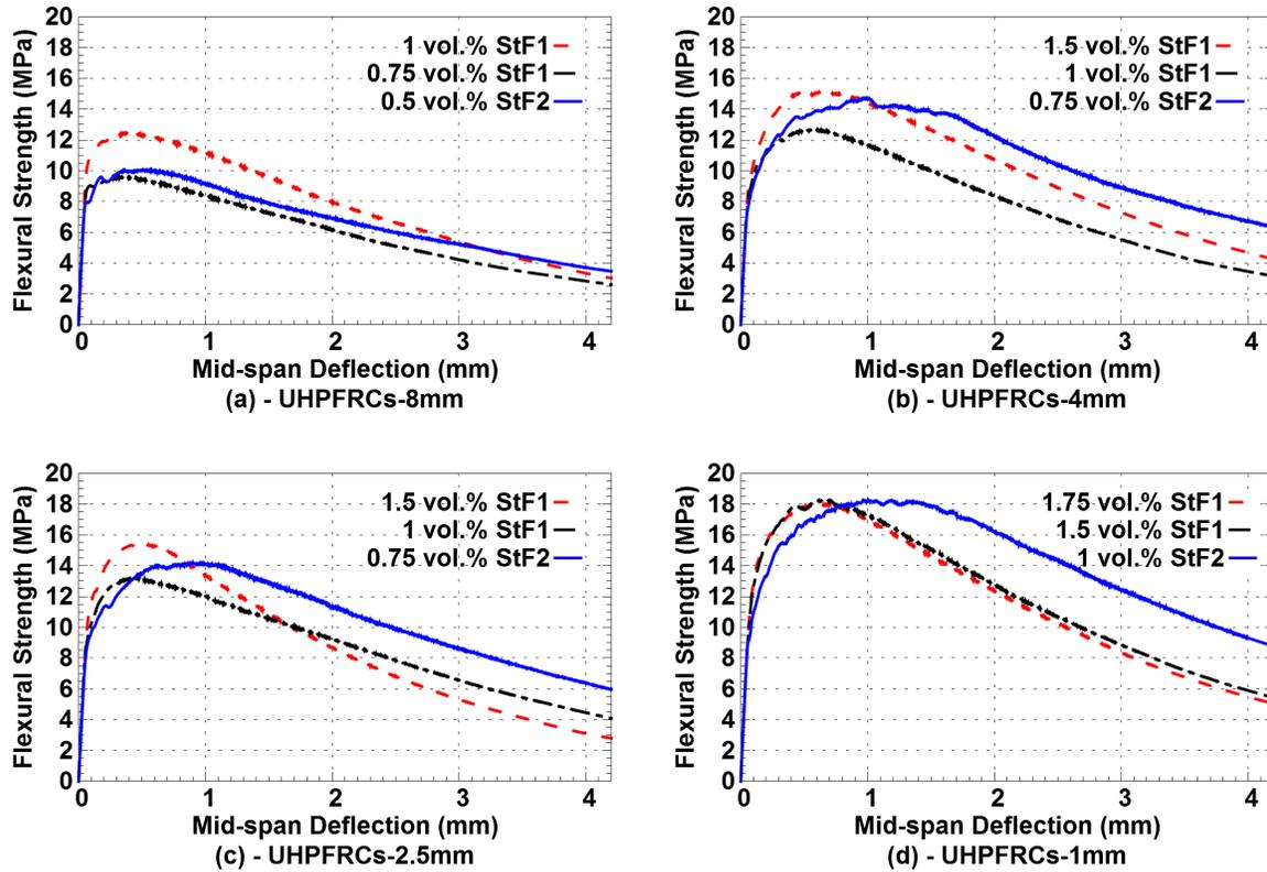
Figure 6: Flexural behaviour of the UHPFRCs based on four-point bending tests using beam of 14x14x56 cm<sup>3</sup>.
