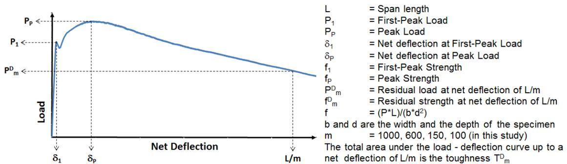
Figure 2: Example of parameter calculations when Peak Load greater than First-Peak Load according to the ASTM C1609/C1609M.
