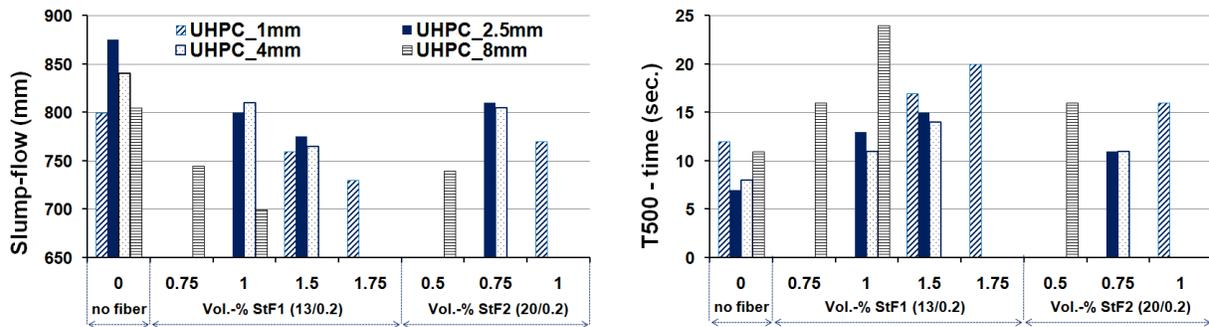
**Figure 4:** The slump-flow (left) and  $T_{500}$  – time (right) of UHPCs with and without fibres, the fibre contents were less than or equal to the critical volume fraction.
