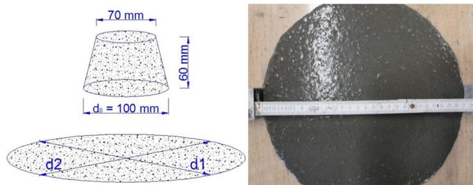
Figure 2: The spread-flow test to evaluate the flowability of fresh concrete using Haegermann cone.
