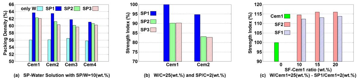
**Figure 3:** (a): The influence of SP on the packing density of the cements using a solution with SP/W of 10 (wt.%); (b): The influence of three superplasticizers on the 28 days compressive strength of Cem.No.1 & 2.; (c): Influence of types and content of silica fumes on the 28 days strength of silica fumes – Cem.No.1 binders.
