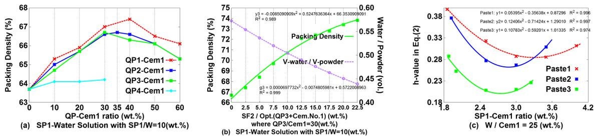
**Figure 4:** (a): Determination of the optimum packing density mixtures of the quartz powders and Cem.No.1; (b): The increase of the packing density of cementitious materials of (QP3+Cem.No.1+SF2) (solid curves) and the decrease of the volume ratio of water to powder in concrete with W/C of 0.25 (dashed curves) by the increasing of SF2; (c): Influence of SP1 content on the plastic viscosity of the cementitious pastes with the W/C = 0.25.
