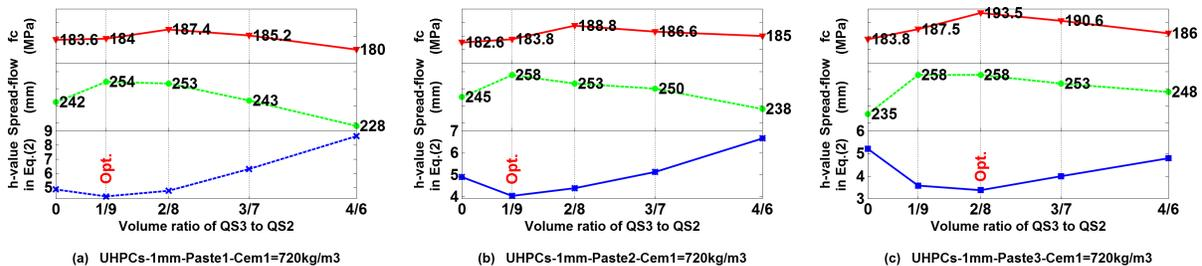
**Figure 5:** Relations between the plastic viscosity, self-flowability, compressive strength of UHPCs\_1mm with different combinations of QS3 and QS2 - (a): Paste 1, (b): Paste 2, (c): Paste 3.
