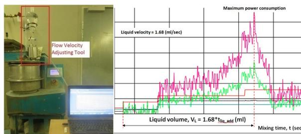
**Figure 1:** The equipment for the superplasticizer-water solution demand test (left), and the development of power consumption during addition of the solution (right).
