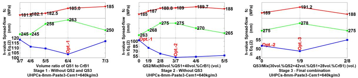
**Figure 6:** The process of the SwOPPD for UHPCs\_8mm-Paste 3-CrB1 & QS1&2&3 (optimum volume ratio QS3/QS2/QS1/CrB1 = 10/27/37.8/25.2).
