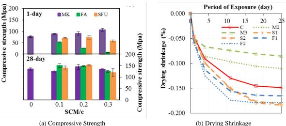
Figure 3. Hardened State Properties of Paste Using Binary Blend of SCM and Cement
