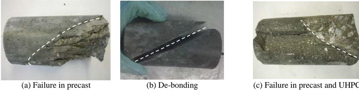
**Figure 2. Failure Modes of Slant Shear Test**
