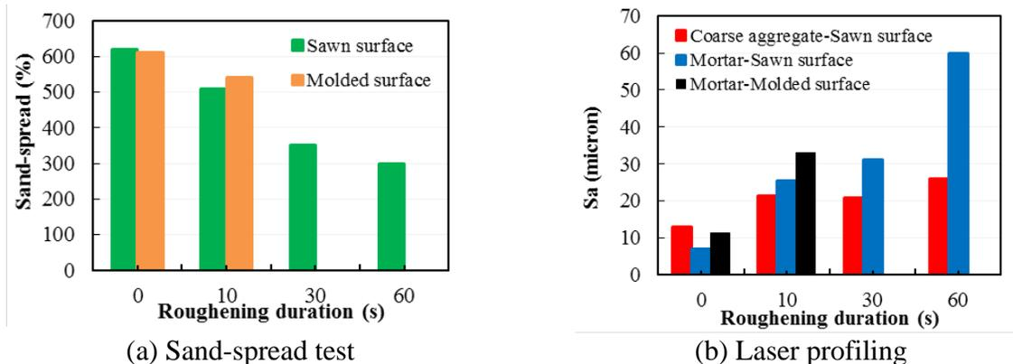
**Figure 3. Influence of Roughening Duration on the Substrate Surface Roughness**
