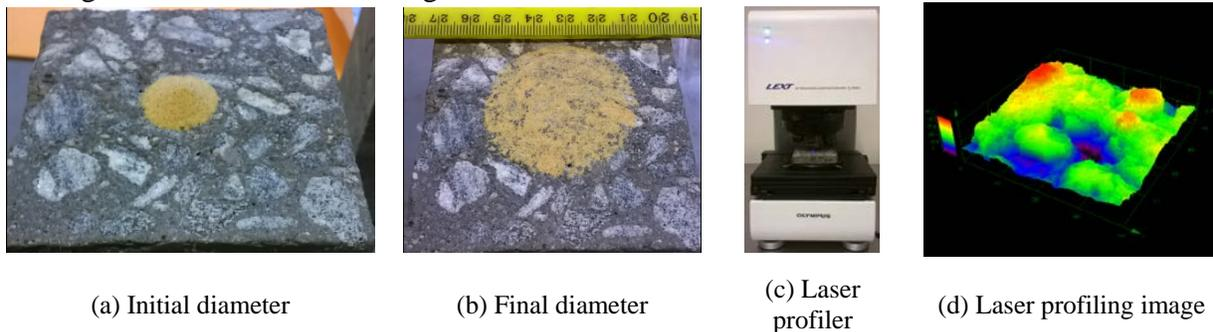
**Figure 1. Sand-Spread Test and Laser Profiling**
