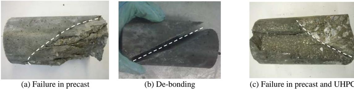
**Figure 2. Failure Modes of Slant Shear Test**
