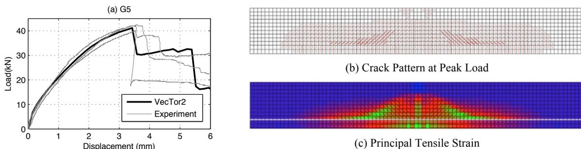
Figure 7. G5 VecTor2 Load-Displacement, Crack Patterns, and Principal Tensile Strain
