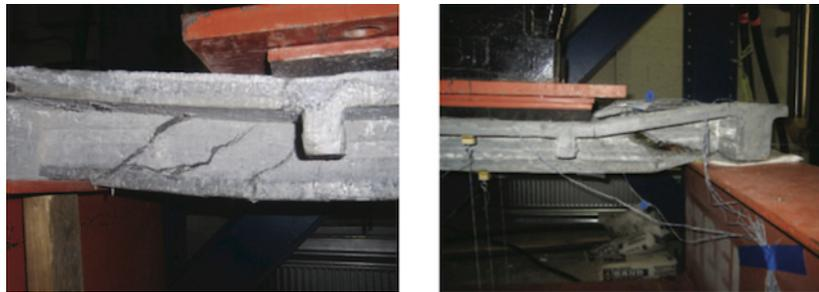
Figure 1. Failure Modes of UHPC-HSS With and Without Stirrups (Xia 2011)
