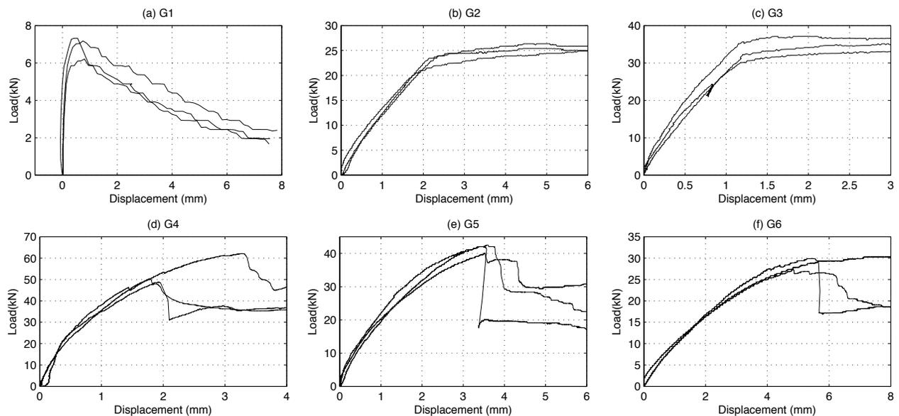
Figure 4. G1-G6 Experimental Load-Displacement
