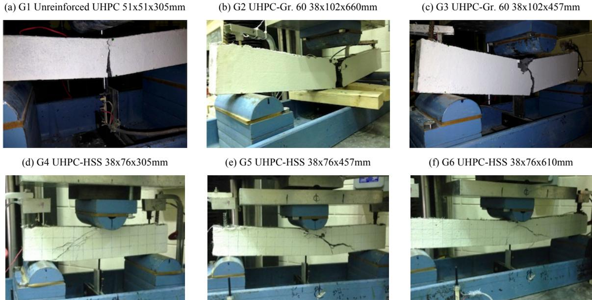
Figure 3. G1-G6 Typical Failure Modes
