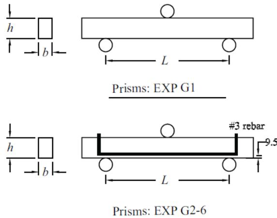
**Figure 2. Specimen Setups**
