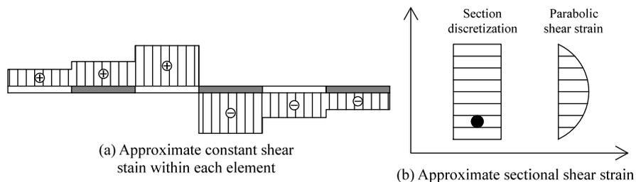
**Figure 5. Approximate Elemental and Sectional Shear Strains**
