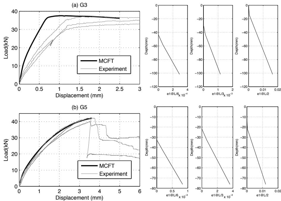
**Figure 6. G3 and G5 MCFT Load-Displacement and Principal Tensile Strain at the Peak**
