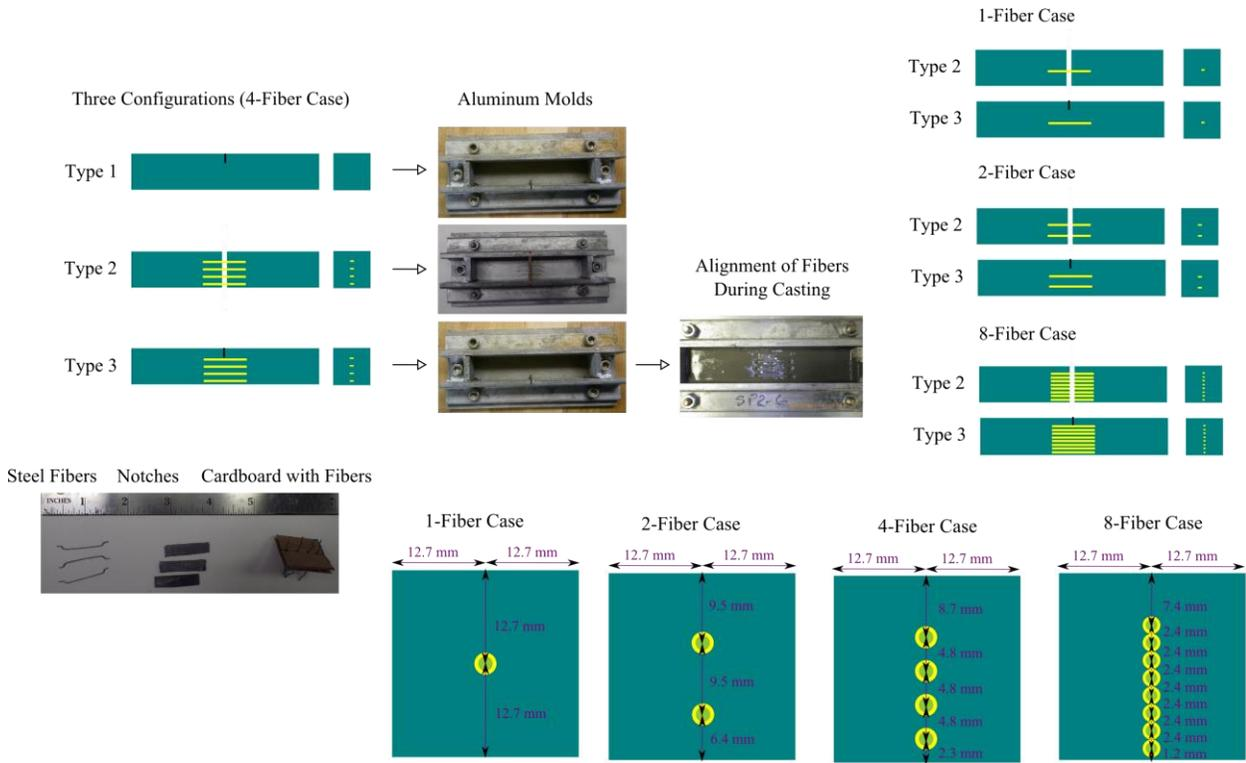
**Figure 1. Three different configurations used in the experiment and the nominal positions of the fibers in each case.**
