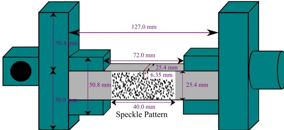
**Figure 2. Dimensions of the specimen.**
