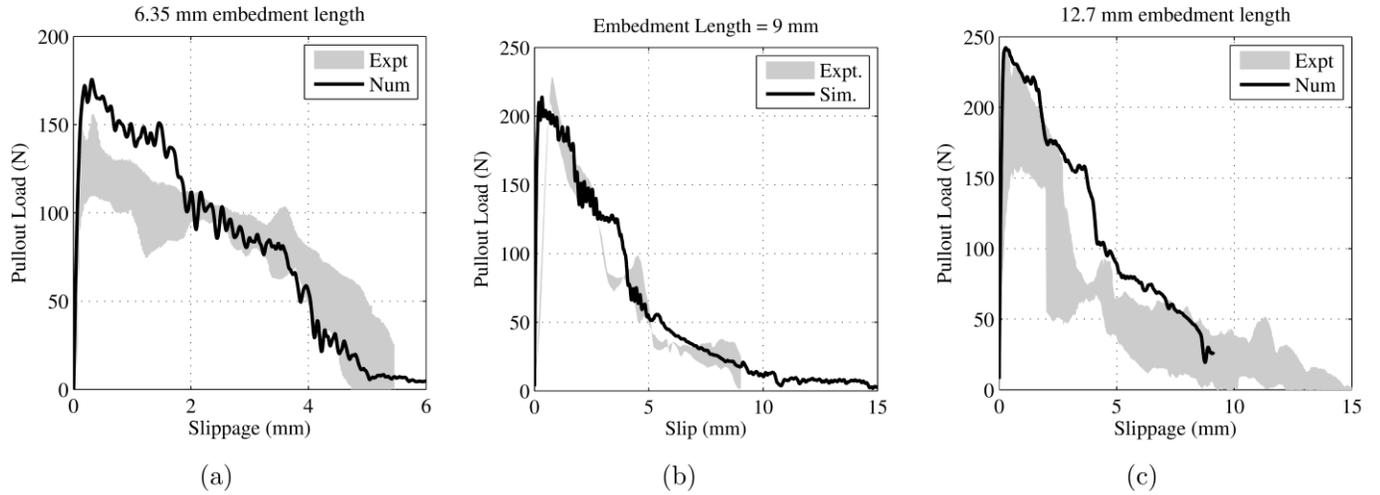
**Figure 6. Effects of embedment length: (a) 6.35 mm embedment length, (b) 9 mm embedment length, and (c) 12.7 mm embedment length.**
