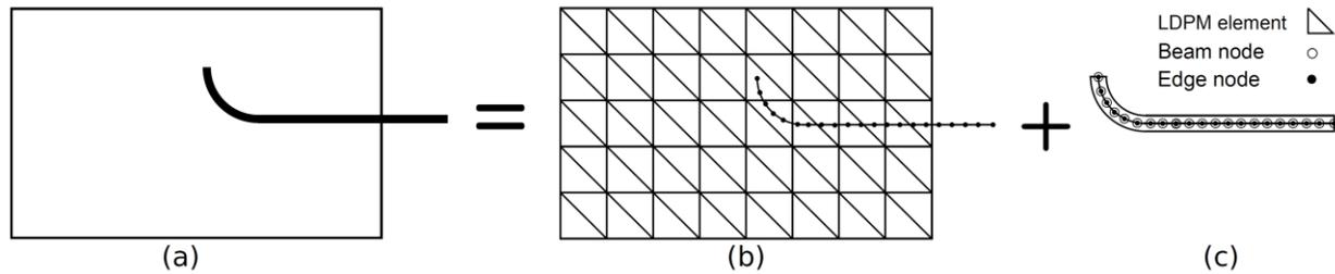
**Figure 5. Kinematic model of fiber pullout test. (a) concrete specimen and fiber; (b) master-slave constraint between matrix (LDPM mesh) and fiber tunnel (geometric edge list); (c) penalty constraint between tunnel edge list and fiber (beam list).**
