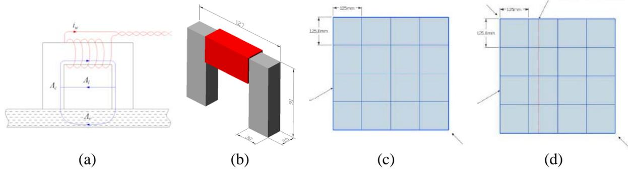
**Figure 3. (a) Scheme of the measurement set-up; (b) employed magnetic probe; schematic cell definition for cell slab without defect (c) and with defect (d).**
