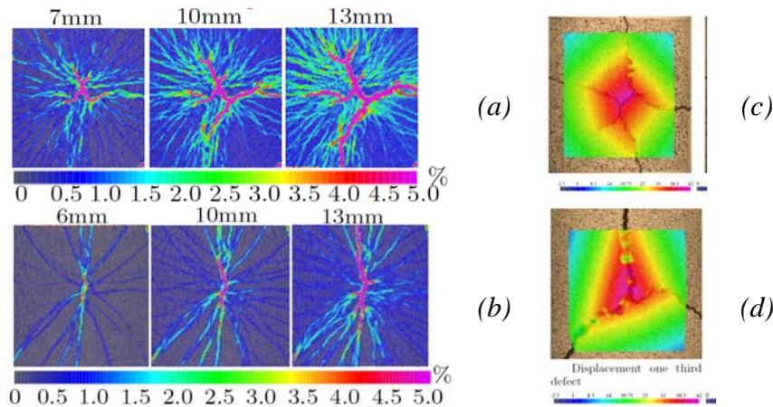
**Figure 6. Crack patterns at different displacement levels for slab without defect (a) and with defect (b). Deflection field at the end of testing: slabs without defect (c) and with defect (d).**
