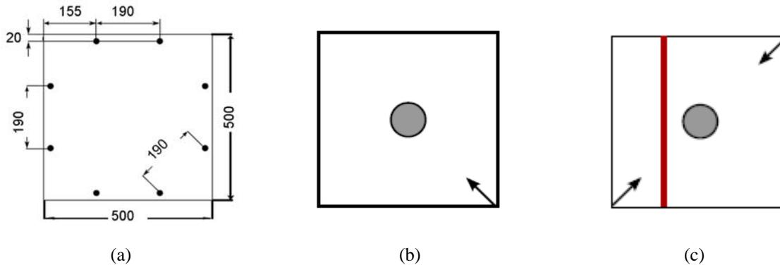
**Figure 2.** (a) Geometry of the UHPFRC slabs (units in mm; 1 mm=0.039 in); (b) slab without defect; (c) slab with casting defect (arrow= casting direction, the grey circle = load).
