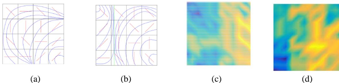
**Figure 4: Direction of maximum compensated inductance and inferred casting flow lines: (a) slab without defect; (b) slab with third side defect. Plots of fractional compensated inductances weighed by local fiber concentration: (c) slab without defect; (d) slab with third side defect.**
