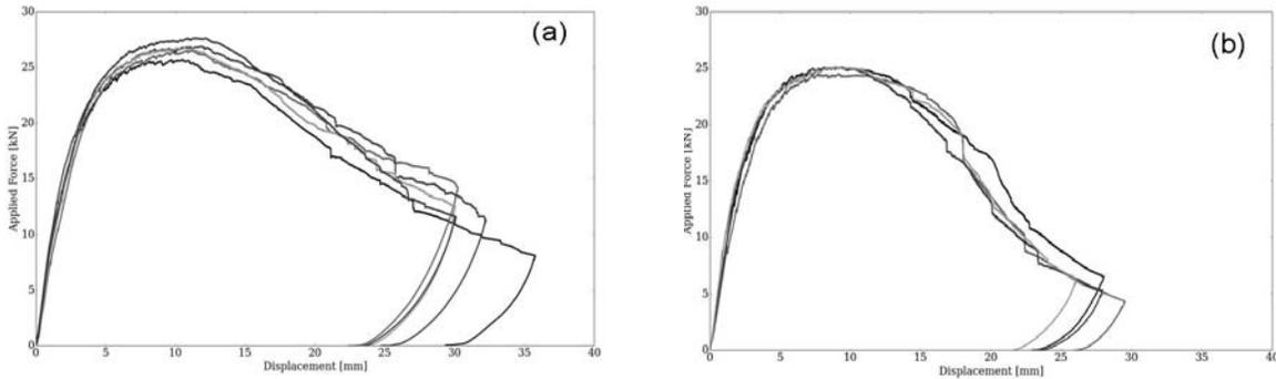
**Figure 5. Load vs. displacement curves for the slabs without defect (a) and the slabs with defect (b).**
