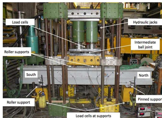
**Figure 3. Experimental testing device of the reinforced UHPFRC beam**
