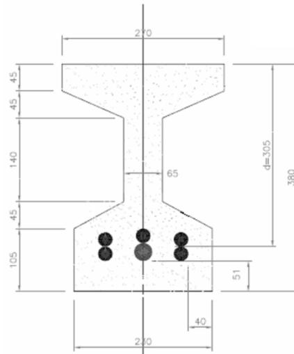
**Figure 2. Cross section of the reinforced UHPFRC beam**
