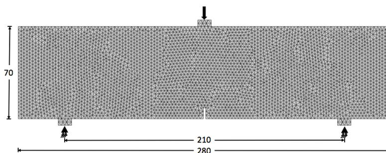
**Figure 4. Finite element mesh of the of notched beams tested in 3-point bending**
