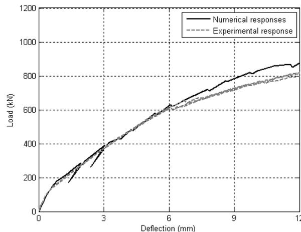
**Figure 9. Experimental and numerical load-deflection curves of the reinforced UHPFRC beam with increased post-cracking energy**
