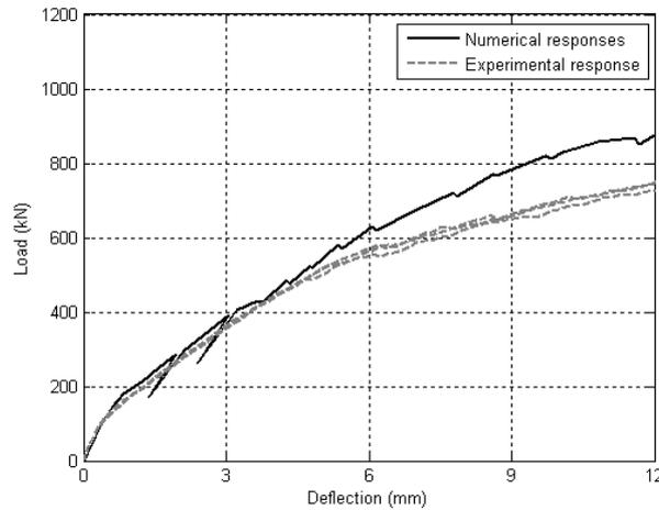
**Figure 7. Experimental and numerical load-deflection curves of the reinforced UHPFRC beam**
