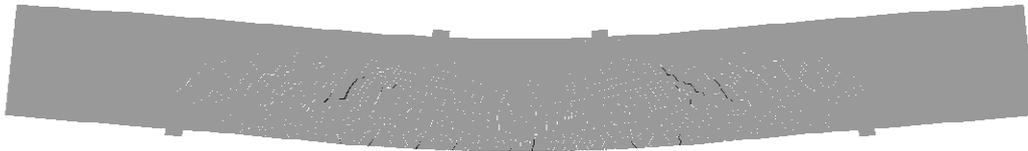
**Figure 8. Example of cracking process of the reinforced UHPFRC beam**
