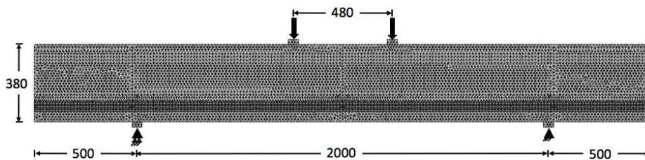
**Figure 6. Finite element mesh of the reinforced UHPFRC beam**
