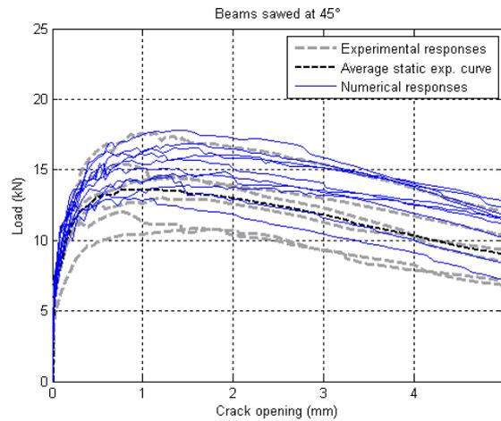
**Figure 5. Experimental and numerical load-crack opening curves of the beams sawed at 45°**
