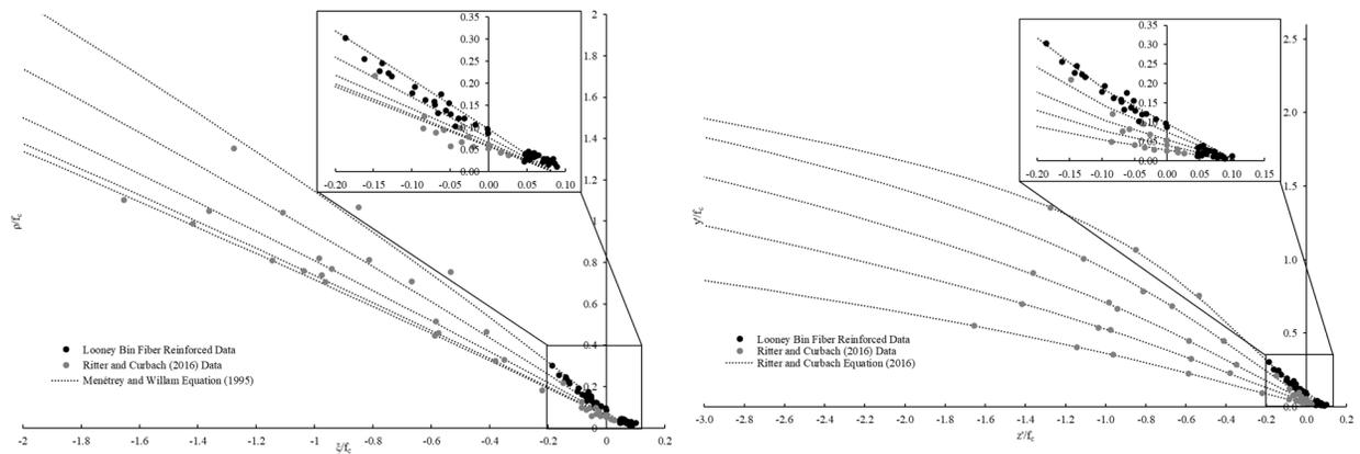
Figure 2 - Menétrey and Willam fit (left) and Ritter and Curbach fit (right)
