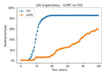
Figure 1. Life expectancy estimation for UHPC and Conventional Concrete.
