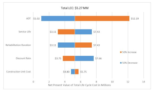
Figure 2. Tornedo diagram for sensitivity analysis of alternative 1.
