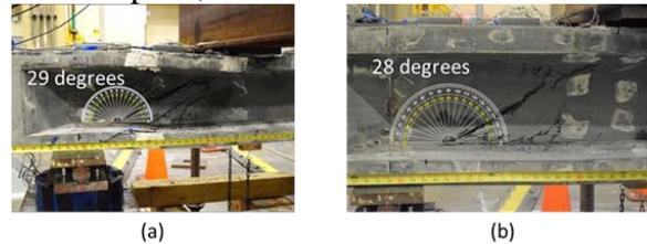
**Figure 7 Condition of UHPC piles after shear testing with crack angles for a) 12-in. pile and b) 14-in. pile**
