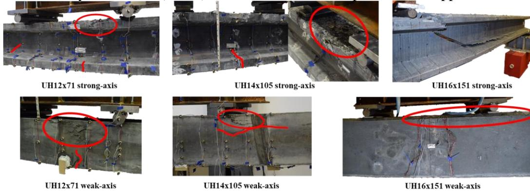
Figure 5 Condition of UHPC piles after flexural testing
