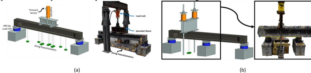
**Figure 3 Experimental schematic and lab test setup for a) flexural testing and b) shear testing**
