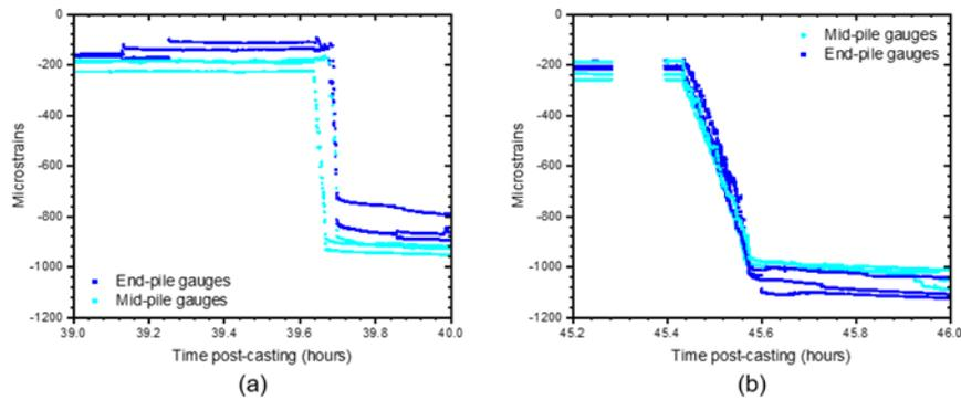
Figure 4 Strain gauge readings in piles during detensioning for a) 12 and 14-in. piles and b) 16-in. piles
