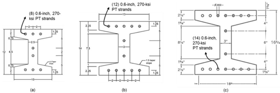
**Figure 1 UHPC Sections: (a) UH12x71, (b) UH14x105, (c) UH16x151**
