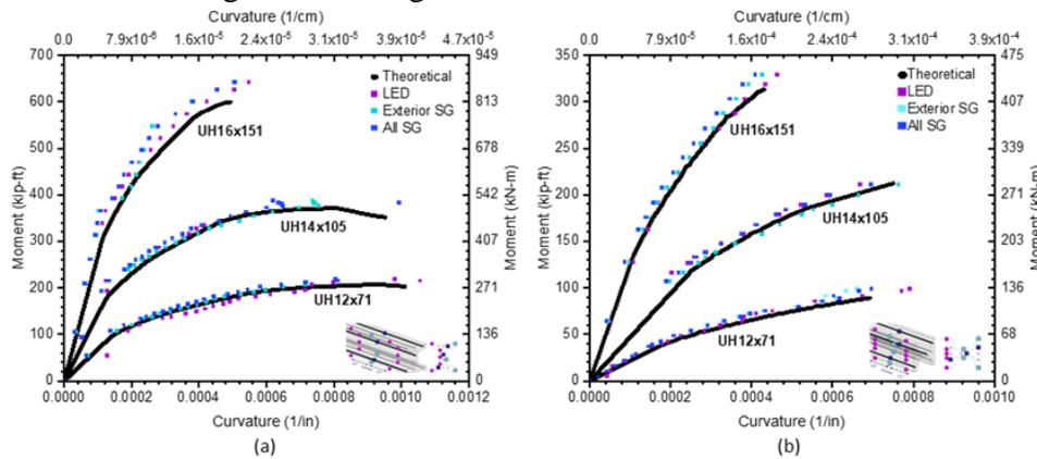
Figure 6 Moment-curvature comparisons for a) strong-axis and b) weak-axis bending
