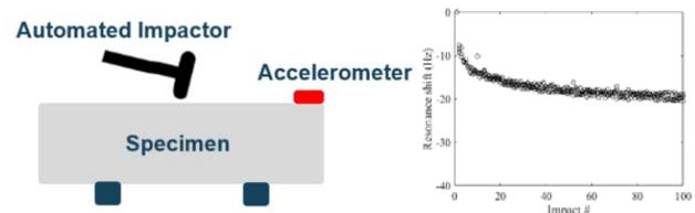
FIGURE 2: SCHEMATIC OF TEST SETUP FOR SDIT AND TYPICAL MEASUREMENT RESULTS
