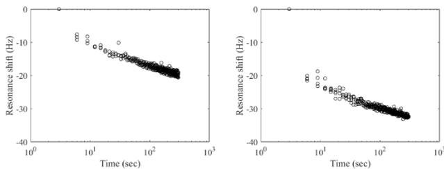
**FIGURE 4: RESONANCE SHIFT VS LOG(TIME) WITH THREE REPEATITIONS ON PRISTINE AND CARBON TREATED BEREASANDSTONE SAMPLE 2**
