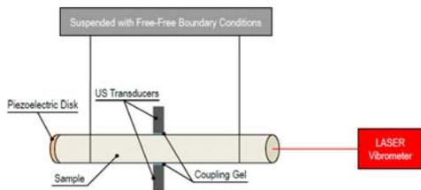
FIGURE 1: SCHEMATIC FOR NRUS
