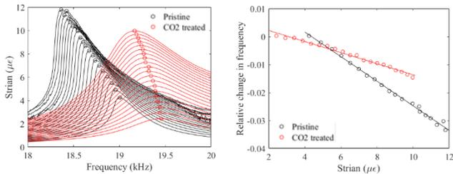
**FIGURE 3: NRUS RESULTS FOR PRISTINE AND CARBON EXPOSED BEREASANDSTONE SAMPLE**
