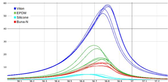
**FIGURE 2: EXAMPLE OVERLAY OF A SMALL SECTION OF THE SPECTRA FOR O-RINGS. COLORS INDICATE MATERIAL TYPE.**
