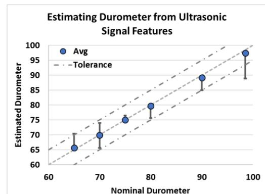
**FIGURE 3: DUROMETER ESTIMATES FOR POPULATIONS OF O-RINGS USING ULTRASONIC SIGNAL FEATURES.**
