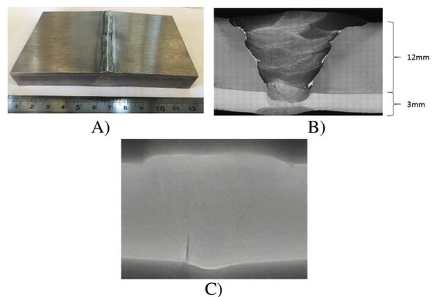
**FIGURE 2:** A) PHOTO OF THE SAMPLE WITH THE FATIGUE CRACK; B) METALLOGRAPHY IMAGE OF THE WELD CROSS SECTION; C) CT CROSS SECTION IMAGE OF THE SAMPLE WHERE THE FATIGUE CRACK CAN BE NOTICED BESIDES THE WELD ROOT.
