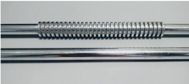
**FIGURE 1:** Photograph of Waveguide metamaterial sample with and without baffles.
