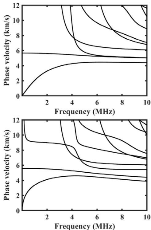
**FIGURE.4** THE DISPERSION CURVES FOR IRON BASED ALUMINA FGM PIPE:  $\eta=4, \eta=100$
