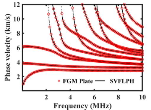
**FIGURE.2** COMPARISON OF THE DISPERSION CURVES FOR IRON BASED ALUMINA BY PIPE AND PLATE
