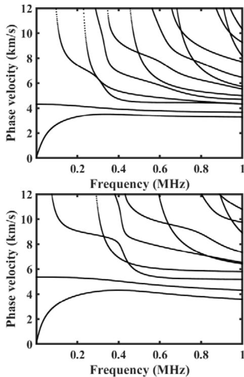
**FIGURE.3** THE DISPERSION CURVES FOR IRON BASED ALUMINA FGM PIPE:  $p=1, p=5$ .
