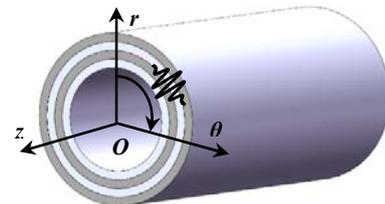
FIGURE 1: THE GEOMETRY OF FGM HOLLOW CYLINDERS
