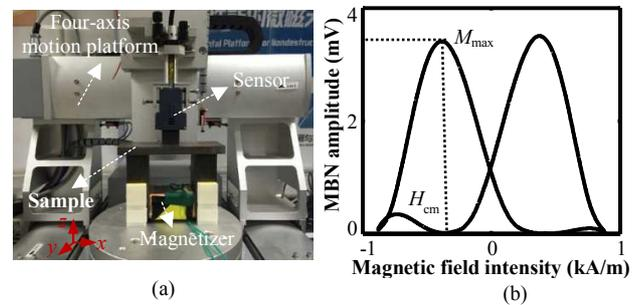
**FIGURE 4:** EXPERIMENTAL SET-UP AND BUTTERFLY MBN PROFILE
