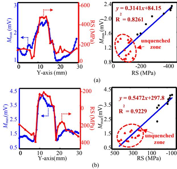
**FIGURE 5:** THE CORRELATION BETWEEN THE PARAMETER OF  $M_{\max}$  AND THE RESIDUAL STRESS
