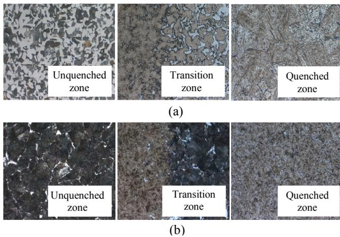
**FIGURE 2:** OPTICAL MICROGRAPHS OF THE MICROSTRUCTURES IN LASER QUENCHING SAMPLE OF (a) 45 STEEL AND (b) 30Cr STEEL
