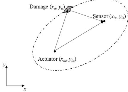
Figure 1. Ellipse method for damage localization.
