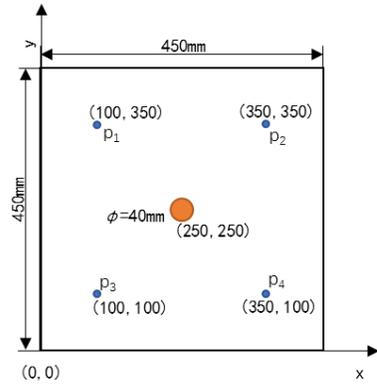
Figure 3. Layout of the composite plate with four PZT transducers in the numerical study.
