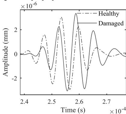
Figure 4. Healthy and damaged time windowed signal of first wave packet for p1-p4 path
