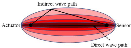
Figure 2. Illustration of the elliptical distribution function of the RAPID algorithm.
