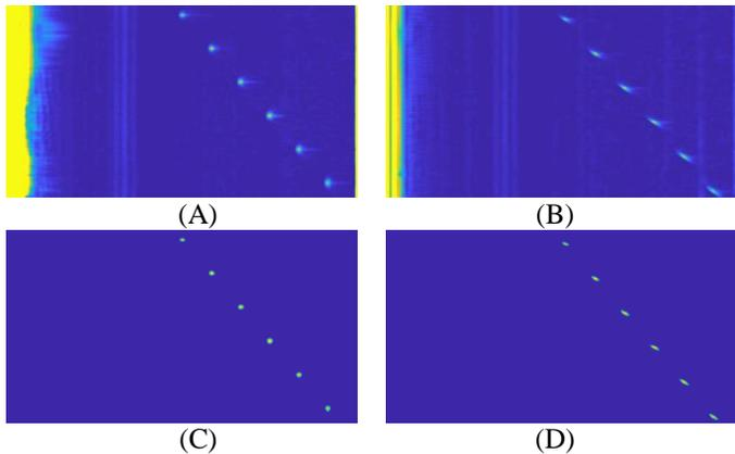
**FIGURE 3:** (A) (B) PHASED ARRAY DATA CAPTURED BY THE BEAM WITH 0 DEGREE AND 10 DEGREE INCIDENT ANGLES AT DIFFERENT LOCATION RESPECTIVELY, (C) (D) FLAW RECOGNITION RESULT FOR THE RAW DATA IN (A) AND (B) CORRESPONDINGLY.
