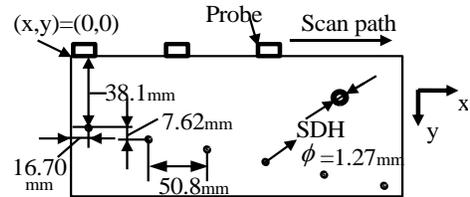
FIGURE 2: A 4340 STEEL BLOCK WITH SIX SDHS
