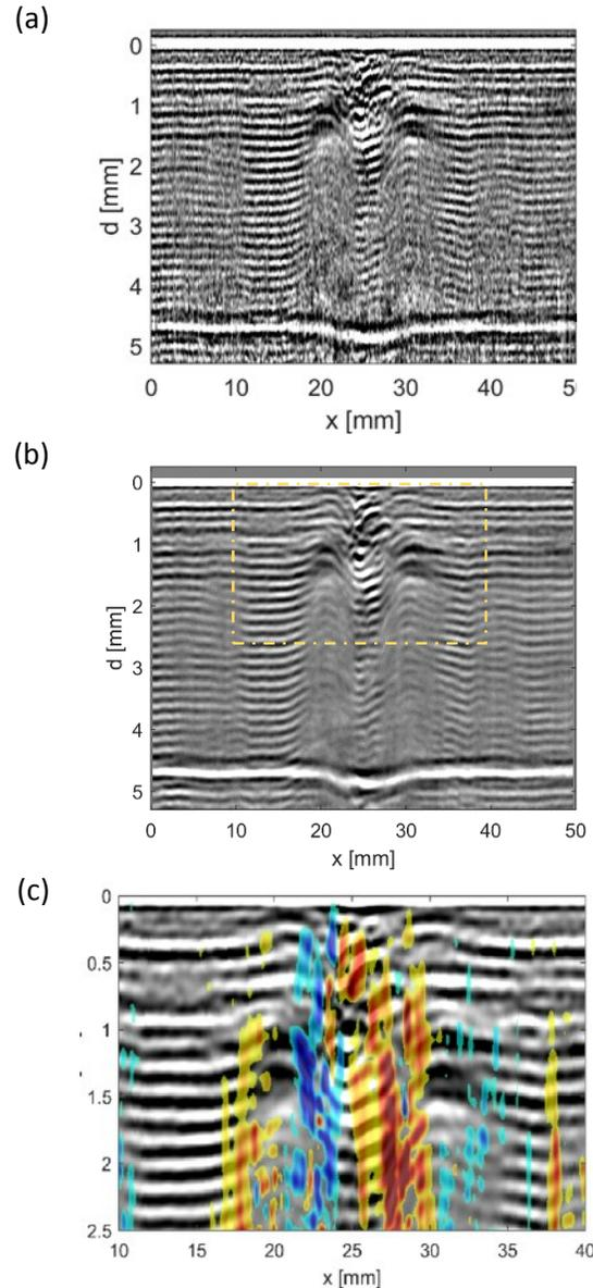
**FIGURE 2:** RAW B-MODE IMAGE OF THE WRINKLED CRFP SAMPLE (a); PROCESSED USING TILT FILTER (b); ZOOMED AREA OF THE PROCESSED IMAGE WITH SUPERIMPOSED LOCAL PLY ROTATION IN DEGREES (c).
