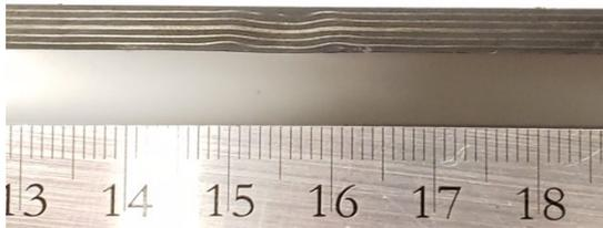
**FIGURE 1:** CROSS-SECTION OF THE WRINKLED AREA OF THE SAMPLE INVESTIGATED IN THIS STUDY.
