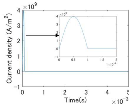
**FIGURE 5:** Profile of exciting current density
