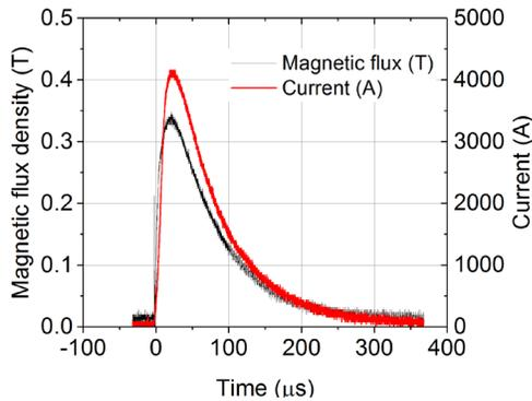
**FIGURE 2:** Magnetic flux density and exciting current [4]
