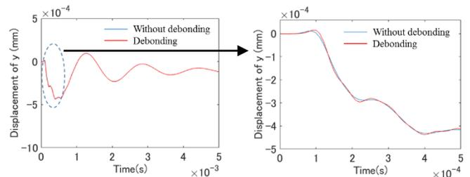
**FIGURE 6:** Simulated vertical displacement at point (0,13.05) in the upper surface of the acrylic plate.
