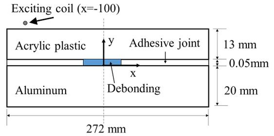
**FIGURE 4:** Geometry of numerical simulation model
