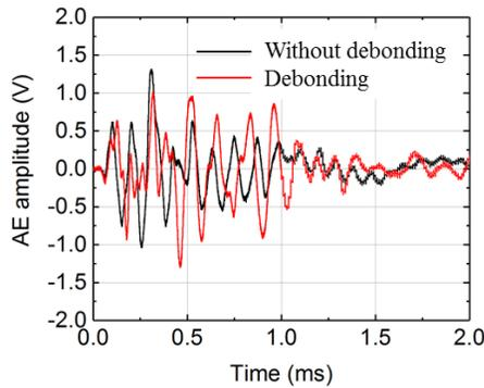
**FIGURE 3:** Received signal from AE sensor [4]
