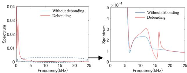
FIGURE 8: Simulated FFT spectrum on vertical displacement at point (0,13.05) in the upper surface of the acrylic plate.
