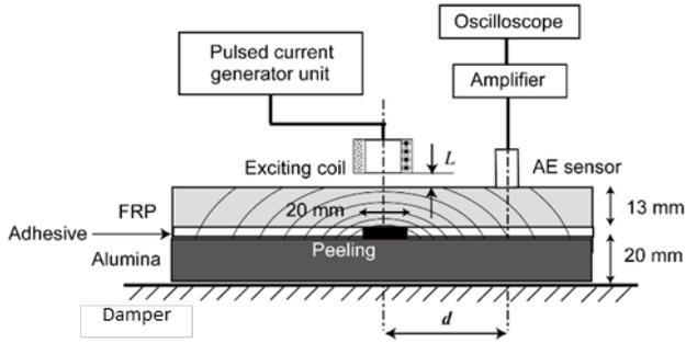
**FIGURE 1:** EPAT system for debonding detection in FRP/Alumina [4]
