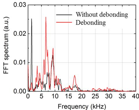
FIGURE 7: FFT spectrum of the received signal from AE sensor
