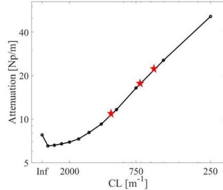
FIGURE 3 : Numerical attenuation curve and experimental values (red stars) - at 500kHz [1]
