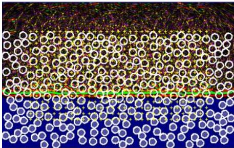
FIGURE 2 : Snapshot of numerical wave propagation: “green/red” color code = P-waves and “yellow/magenta” color code = S-waves [1]
