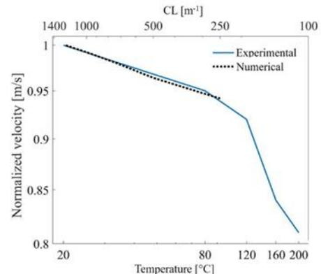
FIGURE 4 : Normalized measured velocities for different levels of thermal damage and numerical velocities for different levels of contact
