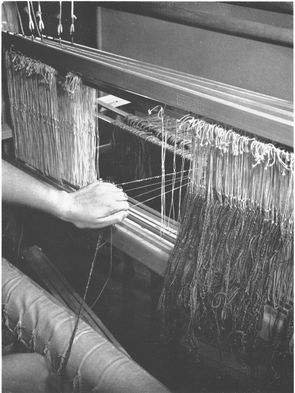
Fig. 6.4—Threading the warp. Yarns are held between the fingers for a simple twill threading. The four yarns are brought forward from the front lease stick without crossing each other. Yarns at right have been threaded through heddles. Warp yet to be threaded can be seen hanging over lease sticks at left. If harnesses were removed to wind the warp onto the warp beam, they have now been hung in place as before.
