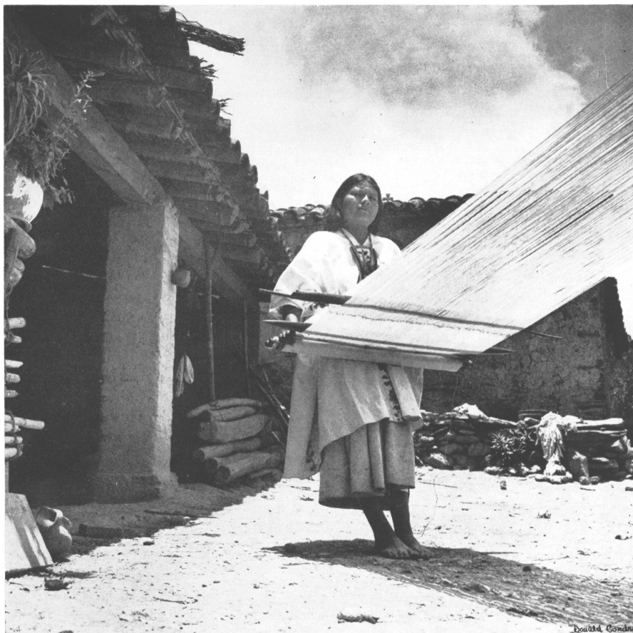
Fig. 1.2—Backstrap loom being used by a Zapotecan woman of Yalalag, Oaxaca, Mexico. (Photograph by Donald Cordry, owned by the Cooper Union Museum. Courtesy "Handweaver and Craftsman.") Tension is maintained by the stance and pull of the body against the loom frame. Length of warp can be increased by wrapping around the upper loom bar, while width is limited by the reach of the arms.
