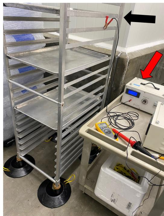
**Figure 1.** A representative image of the experiment setup using the electrostatic thawing system that consists of the electrostatic field generator (red arrow) and a stainless-steel meat cart (black arrow).
