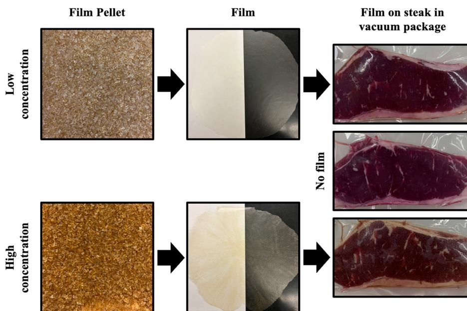
**Figure 1.** Images of color differences between poly(lactic acid) (PLA) film recipes<sup>1</sup>. <sup>1</sup>Low-concentration PLA films were compounded with PLA, 0.12% sodium nitrite, and 0.5%  $\alpha$ -tocopherol, and high-concentration PLA films were compounded with PLA, 0.6% sodium nitrite, and 2.5%  $\alpha$ -tocopherol. PLA films were placed directly on display surface of steaks before being vacuum packaged (Walton's Vacuum Pouch; 10 × 10 pouches; 3 mil thickness).
