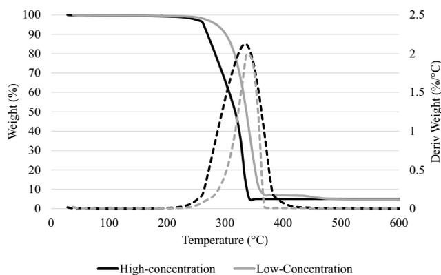
**Figure 2.** Thermogravimetric response<sup>1</sup> of low<sup>2</sup>- and high<sup>3</sup>-concentration poly(lactic acid) (PLA) films. <sup>1</sup>Weight (%) results are given as a continuous line and derivative weight (%/°C) is shown as a dashed line. <sup>2</sup>Low-concentration PLA films were compounded with PLA, 0.12% sodium nitrite, and 0.5%  $\alpha$ -tocopherol. <sup>3</sup>High-concentration PLA films were compounded with PLA, 0.6% sodium nitrite, and 2.5%  $\alpha$ -tocopherol.
