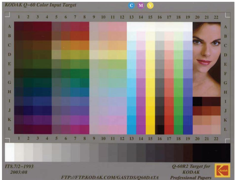
compares the color data generated by the scanner to the known colorimetric values of the pre-measured target (IT8.7/2 Target Q-60 reference data file) to generate the profile.
