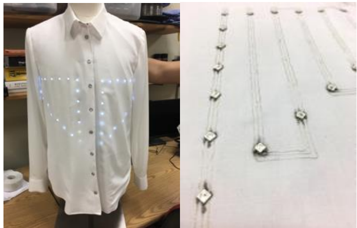
Figure 1. Motion responsive visual display garment, a) final garment, b) Traces and layout for LED display on garment.
