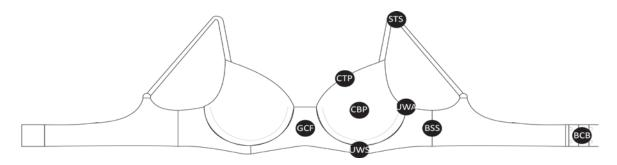
Figure 1. Pressure measurment locations on a bra prototype
