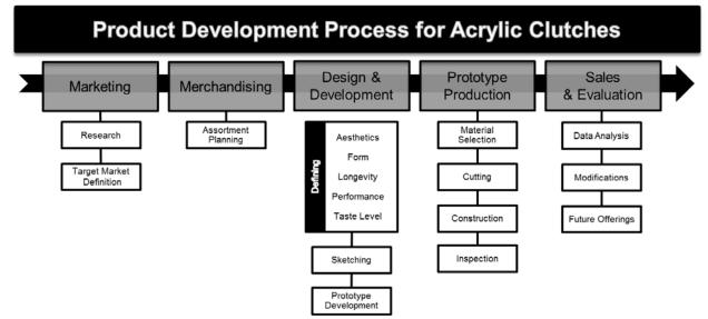
*Figure 1.* Product development process for acrylic clutches adopted from *No-Interval Coherently Phased Product Development Model for Apparel* (May-Plumlee & Little, 1999)
