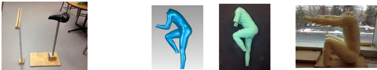
**Figure 1:** Adjustable seat and handlebars for scanning, 3D model in cycling position, form made from sliced foam, symmetrical form.
