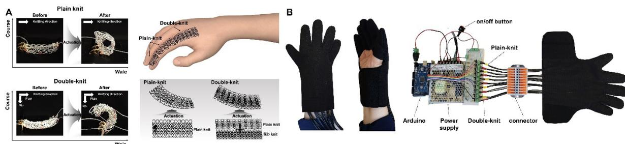
Fig. 1. Exo-glove: A. actuation motion and application method of knitted SMA and B. prototype.
