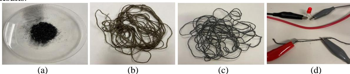
Figure 1: (a) GO Powder, (b) GO coated hemp yarn, (c) rGO Coated hemp yarn, (d) rGO coated hemp yarn conductivity vis connecting LED.
