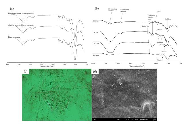
**Figure 1.** (a) ATR-FTIR spectra of alkaline and enzyme pretreated hemp agrowaste, (b) ATR-FTIR spectra of prepared CNCs, (c) OM and (d) SEM images of CNC-alk
