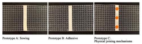
presents the final 3D printed fabric samples: (a) Prototype A: Sewing two 3D printed panels with 12.7mm width of crosssectional areas; (b) Prototype B: Page 1 of 3
