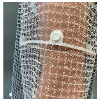
Figure 3. 3D printed snap button
