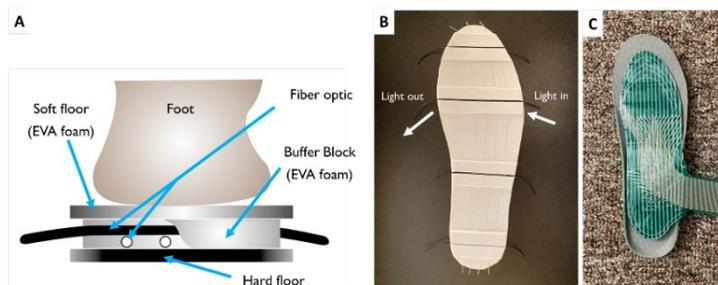
*Figure 1.* (a) Structure and design of the insole, (b) Sensor arranged on the insole, (c) Test setting.
