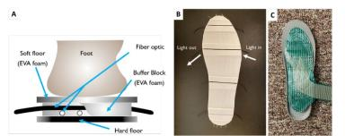
*Figure 1.* (a) Structure and design of the insole, (b) Sensor arranged on the insole, (c) Test setting.
